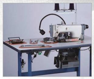
The 84-50 is the lowest priced version in the range of autojig machines and is **ideal for small component pieces with a sewing range up to 30 cm** such as pocket flaps with or without fullness, cuffs, double epaulettes, waistband extension. This model is not equipped with a microprocessor.
