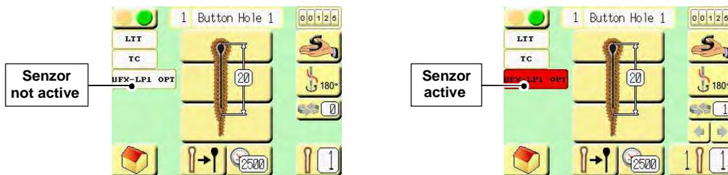
Change of the buttonhole type is shown on the display once the foot pedal is pressed down – see picture. 2:
