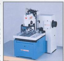
Selection of Buttonhole Cutting (cut before, cut after or no cut) is simply and quickly done by using two levers.
