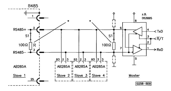
\* = Jumper S1 for terminating resistors
