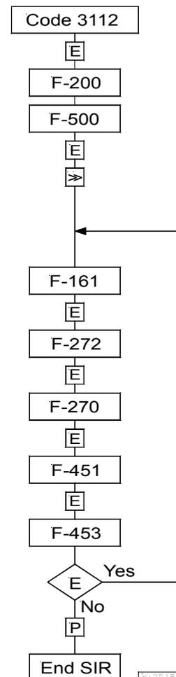
The values can be varied by pressing the +/- keys. When the parameter is displayed on the V810 control panel, press the E key once more for the value to be displayed.
