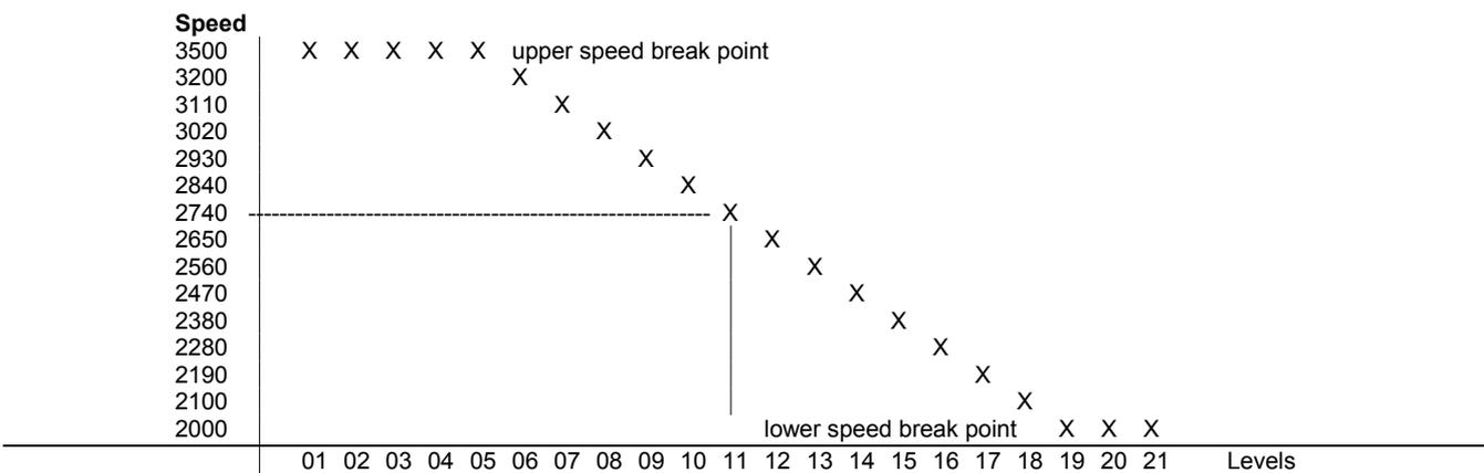
Display example of parameter 188 on the V820 control panel:
