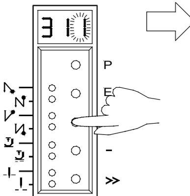
8. Press the E key; the parameter number is displayed, which is indicated by points between the digits.
