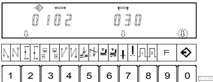
Display of seam **02** after correct function input
