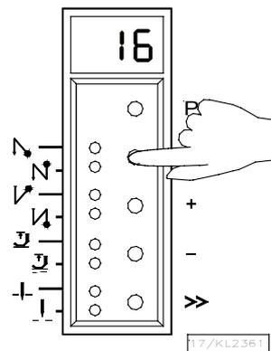
The routine is repeated after pressing the E key. Exit the routine after pressing the P key once. The next parameter number is displayed. Exit programming after pressing the P key. The drive is again ready for sewing.
