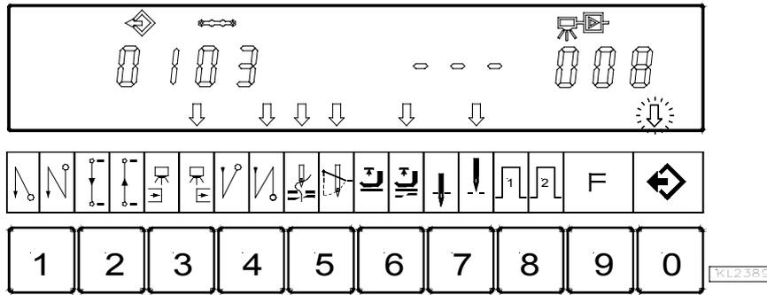
Display of seam **03** after correct function input
