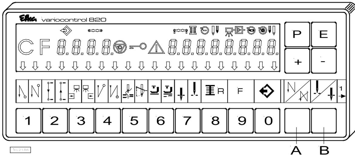
The V820 control panel is supplied with slide-in strip **no. 1** above the keys. For different functions the strip can be replaced with another one supplied with the control panel. Set parameter **292** in this case. See also **V810 / V820** instruction manual!
