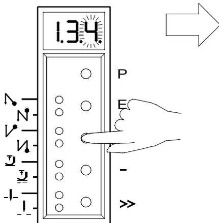
8. Press the E key; the parameter value is displayed. There are no points between the digits.
