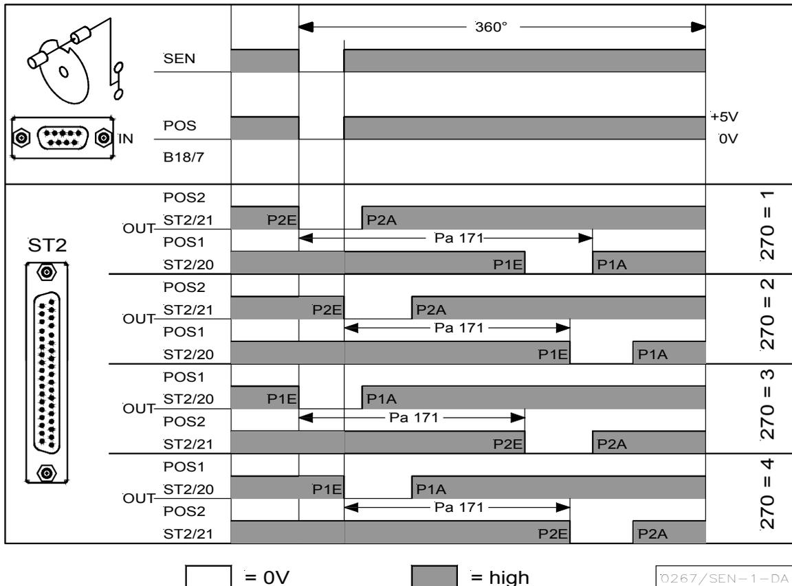
Connection of a sensor e. g. light barrier or proximity switch to socket B18/7. The following settings are possible using parameter 270:
