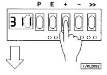
8. Press pushbutton E; the parameter number is displayed, which is indicated by points between the digits.
