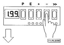
4. After pressing pushbutton E, the parameter value is displayed
