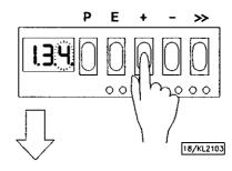
8. Press pushbutton E; parameter value is displayed. There are no points between the digits.
