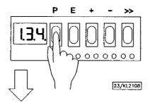
Press pushbutton P. Exit programming. The changed parameter values will only be saved by starting to sew again!
