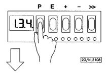
Press pushbutton P. Exit programming. The changed parameter values will only be saved by starting to sew again!
