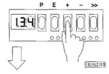
8. Press pushbutton E; parameter value is displayed. There are no points between the digits.
