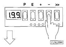
After pressing pushbutton E, the parameter value is displayed
