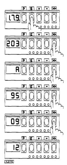
The routine is exited by pressing pushbutton P twice. The drive is again ready for sewing. When pressing pushbutton E, the routine is as well exited, and the next parameter number is displayed.
