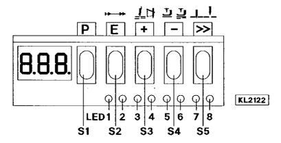
Switchable functions can be changed by pressing a pushbutton. The switching state is indicated by light emitting diodes (LED). See above illustration!
