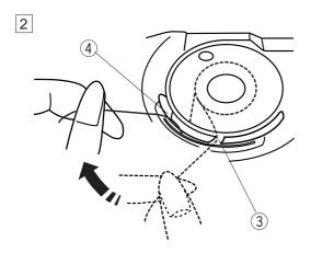
2 Guide the thread into the notch on the front of the bobbin holder.
