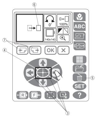
The editing window shows the relative size and placement of the pattern with a square block ⑥ instead of the pattern image.
