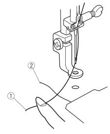
Turn the handwheel one complete turn towards you. Draw the needle thread to bring up a loop of the bobbin thread.
