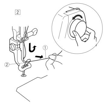
2 Turn the handwheel one complete turn toward you. Draw the needle thread to bring up a loop of the bobbin thread.
