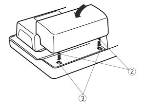
To attach, position the tabs on the base tab holes and push down gently.
