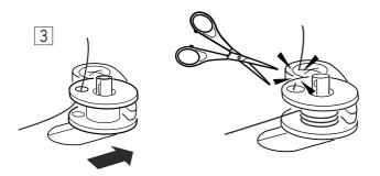
3 Push the spindle to the right. Press the Start/Stop button while holding the end of the thread. Stop the machine after the bobbin has made a few turns. Cut the thread close to the hole in the bobbin.
