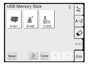
The designs contained in the selected folder will be displayed on the **Pattern selection** keys. Press the **Pattern selection** key to select the desired pattern.
