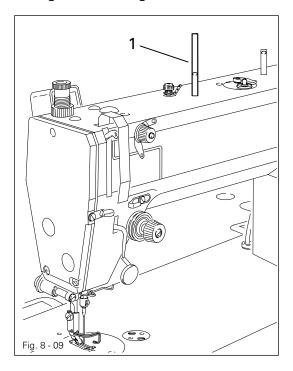
Fit the tapered thread guide pin 1 into the corresponding hole in the machine housing.
