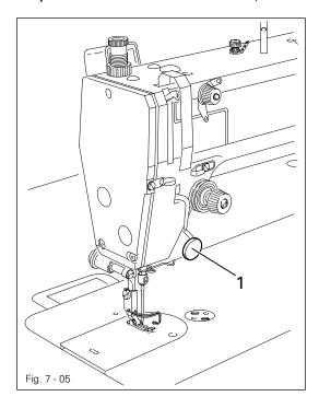
As long as key 1 is pressed during sewing, the machine sews in reverse.
