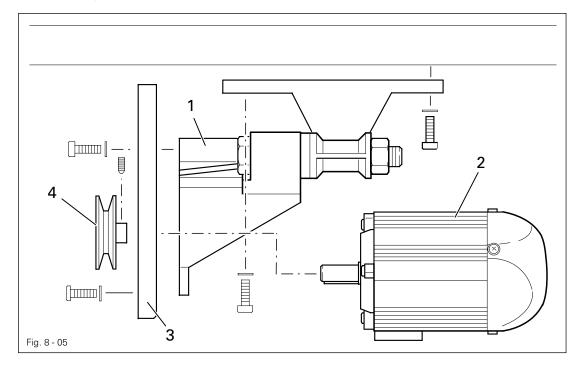
Assemble motor mounting 1, motor 2, belt guard support 3 and belt pulley 4 as shown in Fig. 8-05.
