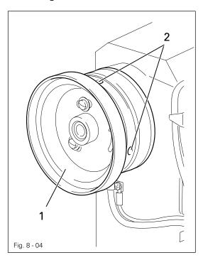
Fit balance wheel 1 and fasten it with 2 screws 2.
