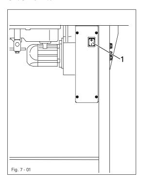
• Switch the machine on or off by turning main switch 1.
