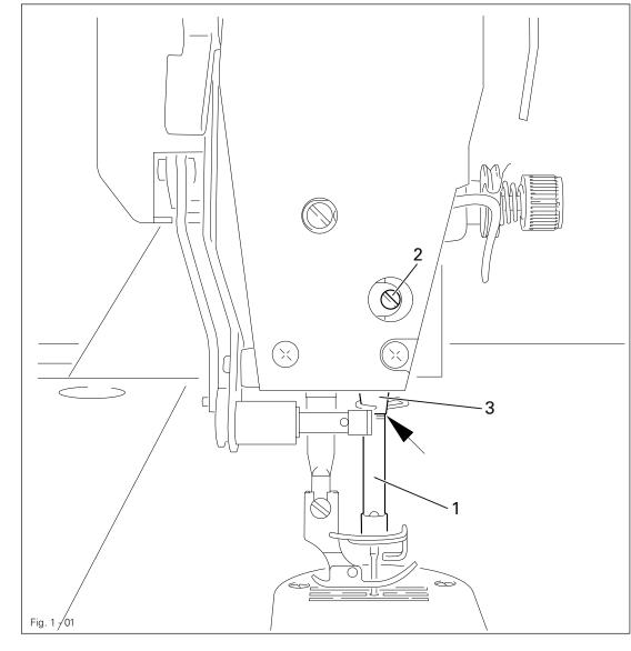
By turning the balance wheel, bring the needle bar to its b.d.c.
