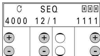
In the sequence mode, the number of programs belonging to the sequence are shown on the display together with the current program. It is possible to switch from one program to another manually with the corresponding **plus/minus** key.
