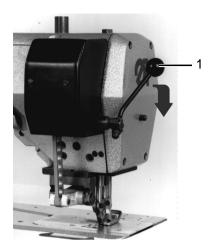
The edge trimmer off CI. 195-671110 may be actuated at any time. It's upper knife is such as formed that also a save cutting aktion is achieved at activating while sewing.
