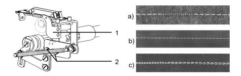
The thread take-up 1 provides for an automatic adjustment of the thread quantity to the set stitch length.
