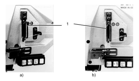
With elastic sewing threads, e.g. synthetic fiber threads, a certain needle thread quantity must be pulled out for sure stitch formation.
