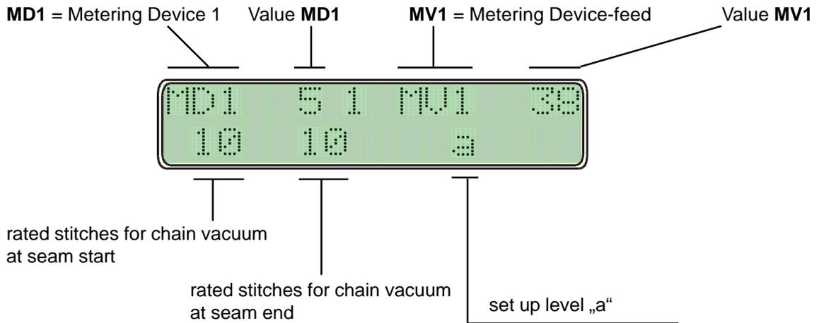
If key ESC is activated (LED is bright), settings for the values from the **MD1** with a range from 0-99 can be made with keys **D+** / **D-** and the settings for values from the **MV1** with a range from 0-999 can be made with keys **L+** / **L-**
