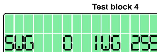
This test block permits to check the synchronizer (increment encoder). For this purpose, the shaft of the motor is rotated manually.
