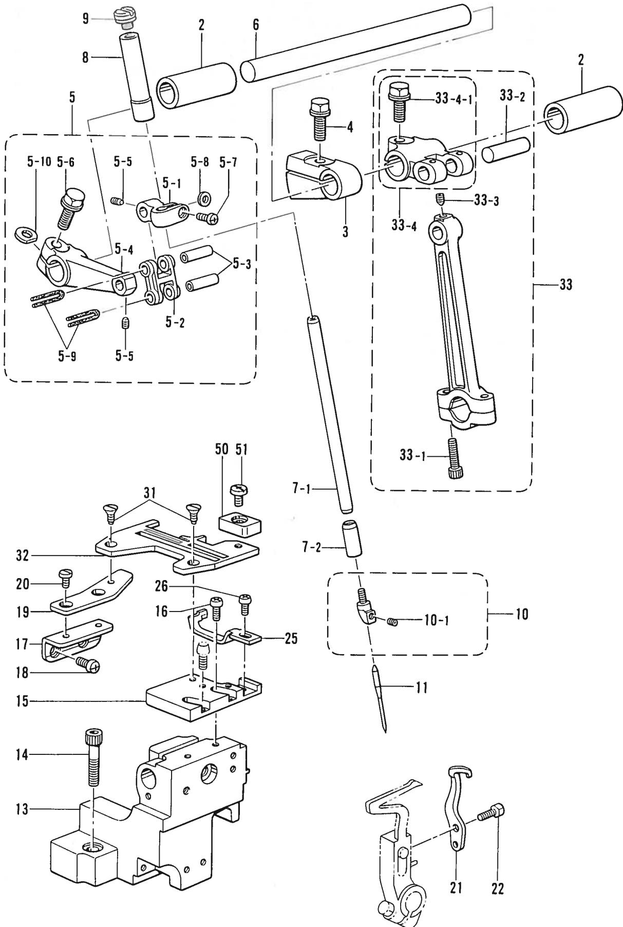
C. 針棒関係/Needle bar mechanism/Nadelstangenvorrichtung/
