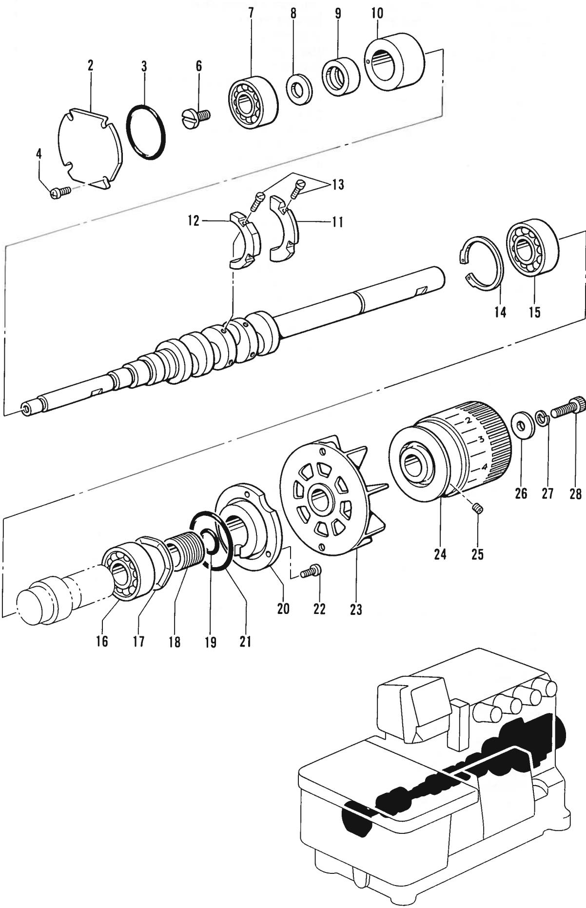
B. 駆動軸関係 / Crank shaft mechanism / Kurbelwelle /
