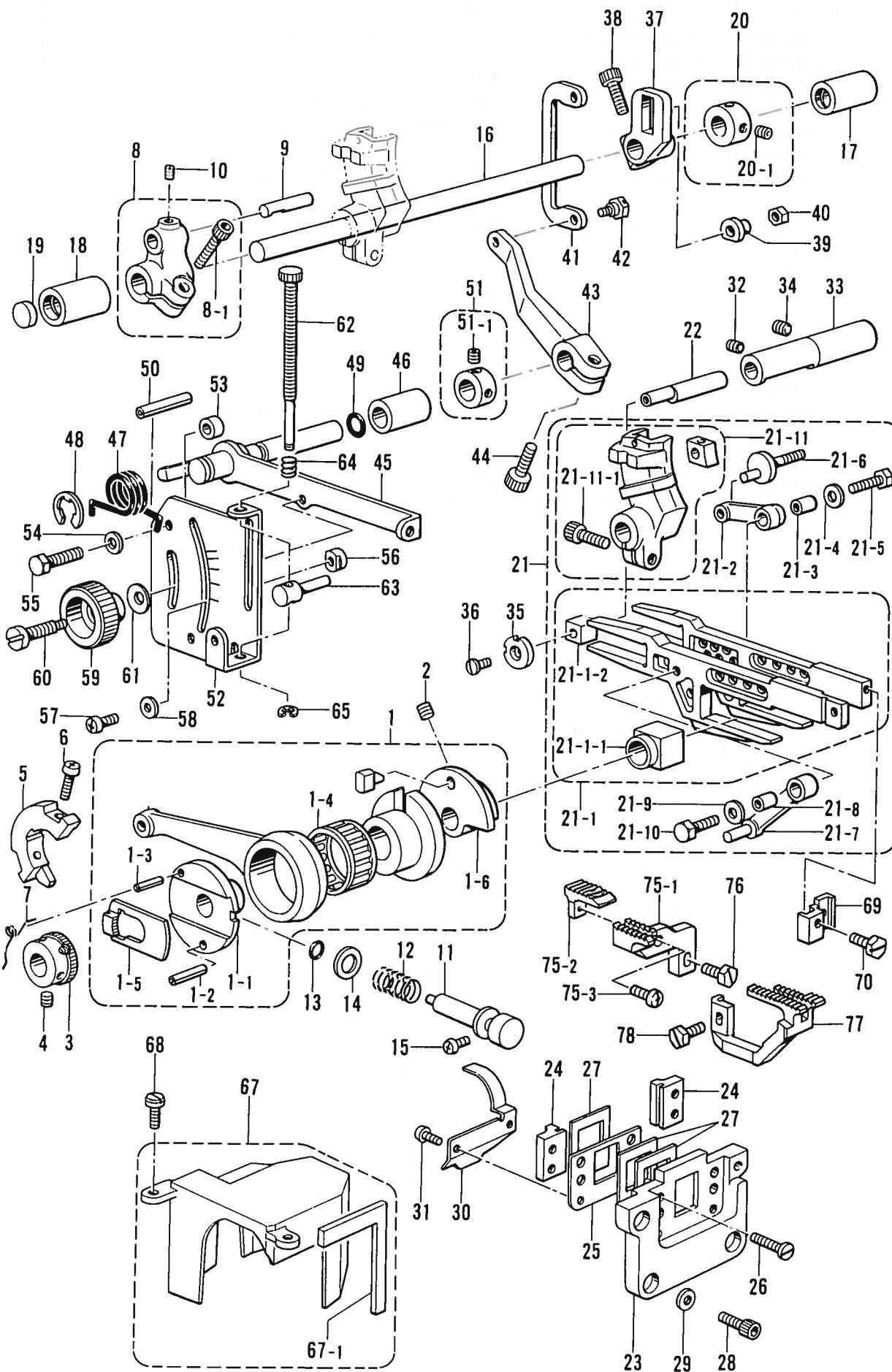
E. 送り関係/Feed mechanism/Transportvorrichtung/
