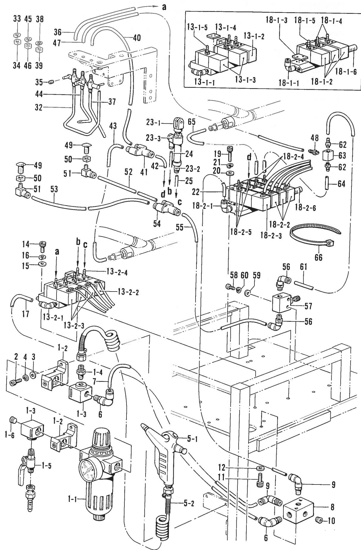
P. 空圧関係/Air pressure mechanism/Luftdruck/
