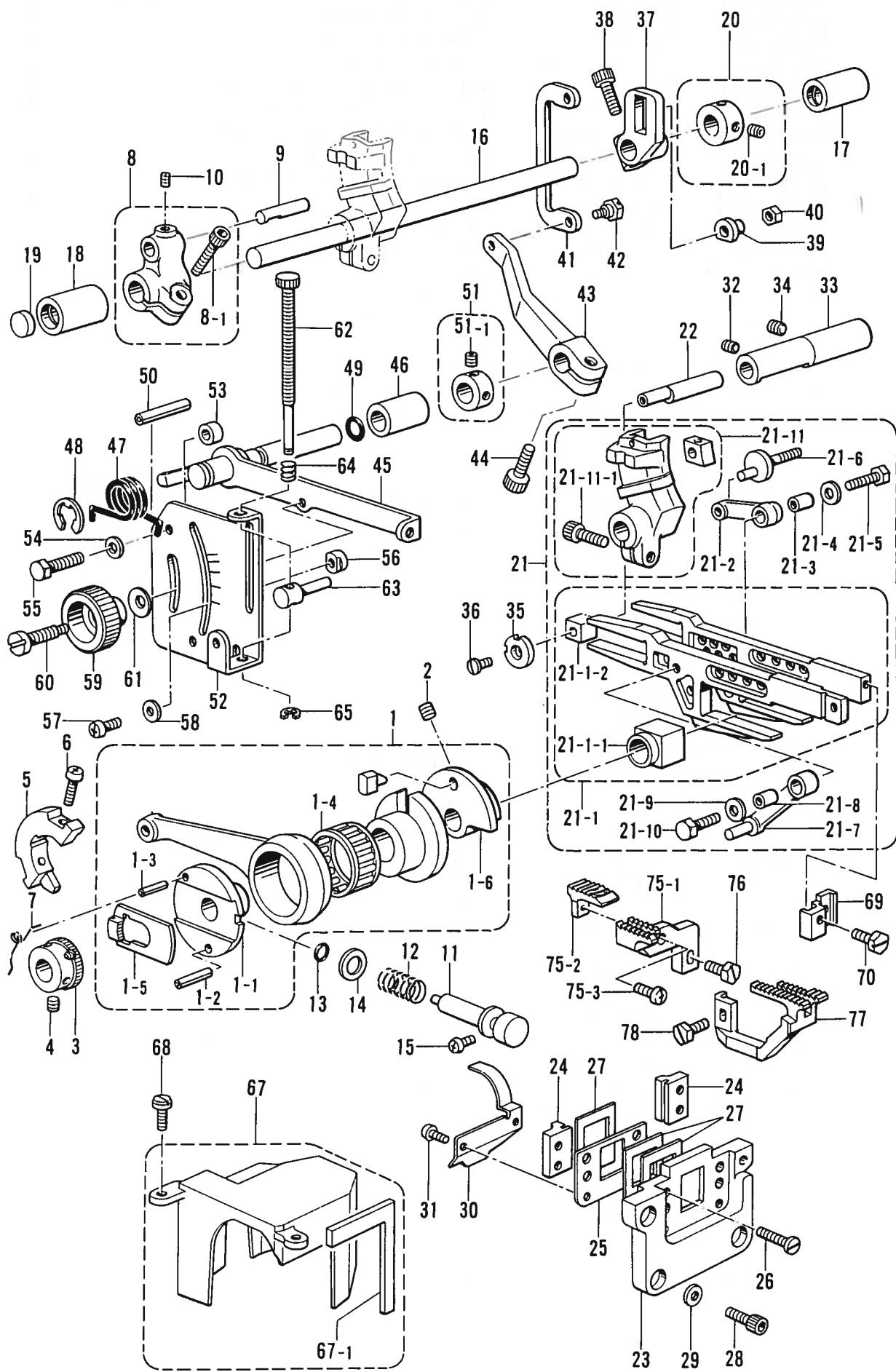
E. 送り関係/Feed mechanism/Transportvorrichtung/
