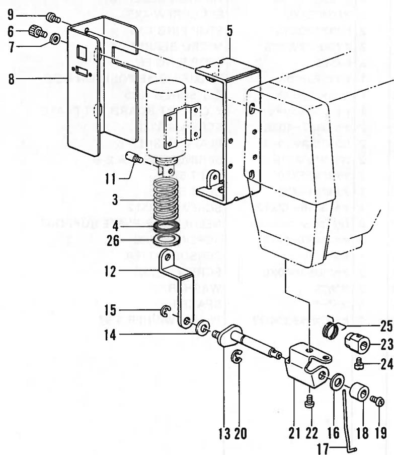
D3. 送り関係 / Feed mechanism / Transportvorrichtung /
