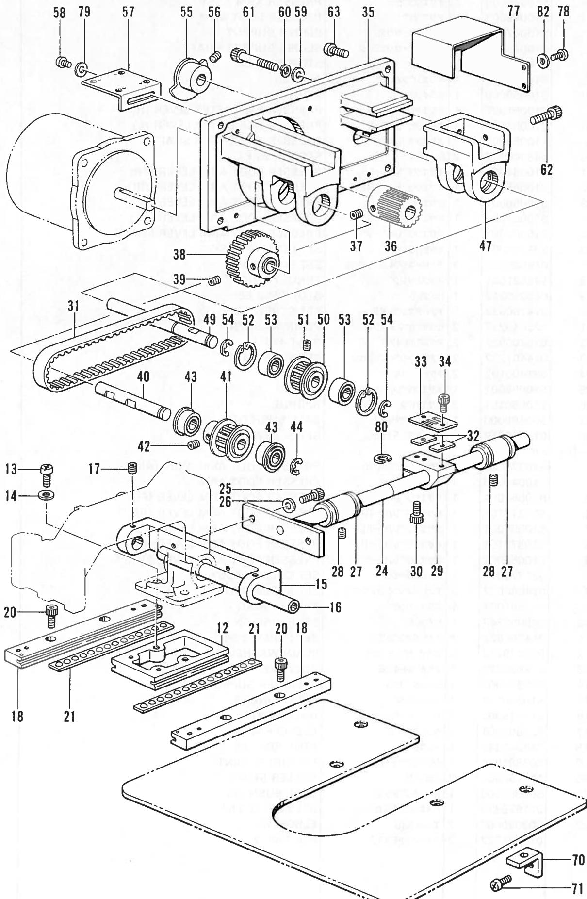
D2. 送り関係/Feed mechanism/Transportvorrichtung/
