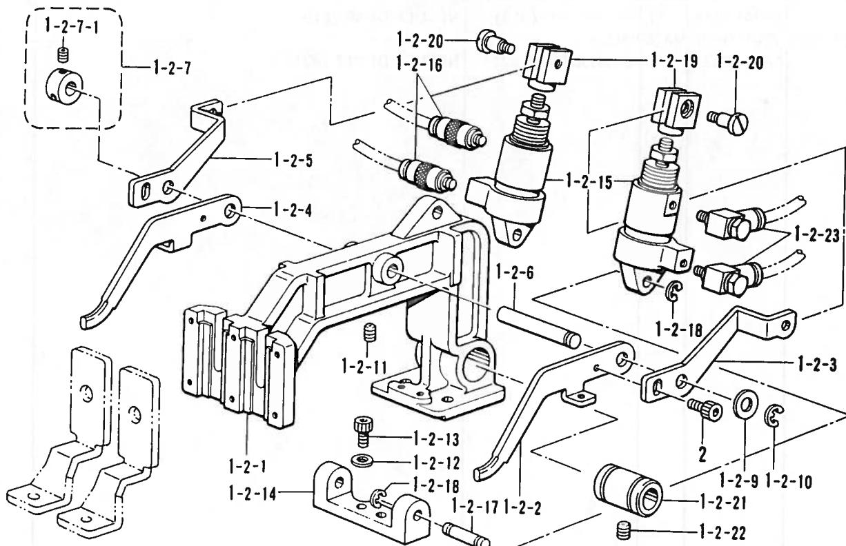
D1. 送り関係 /Feed mechanism/Transportvorrichtung/
