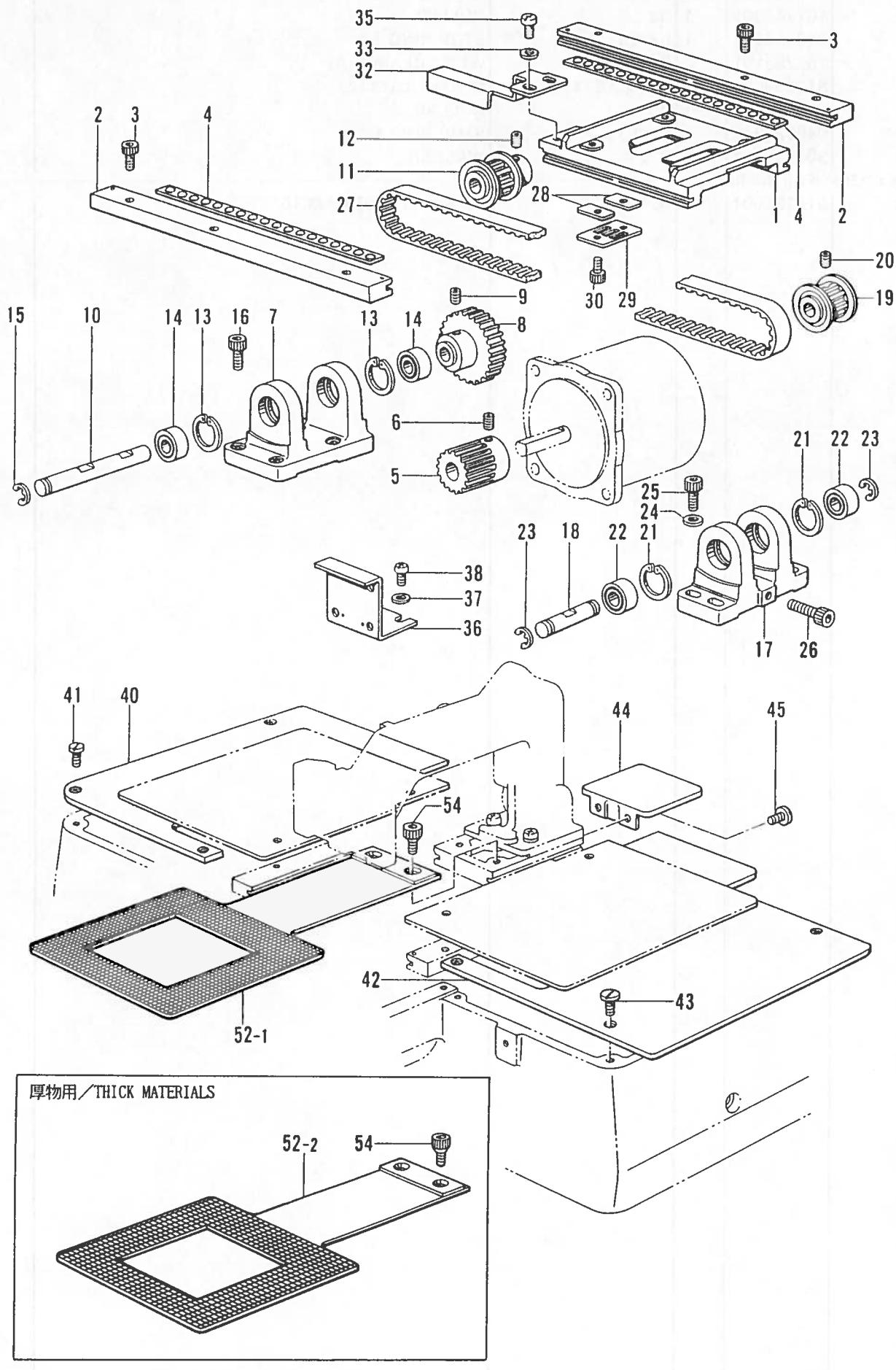
G. 駆動側・送り関係 /Feed guide mechanism/Transportführung/
