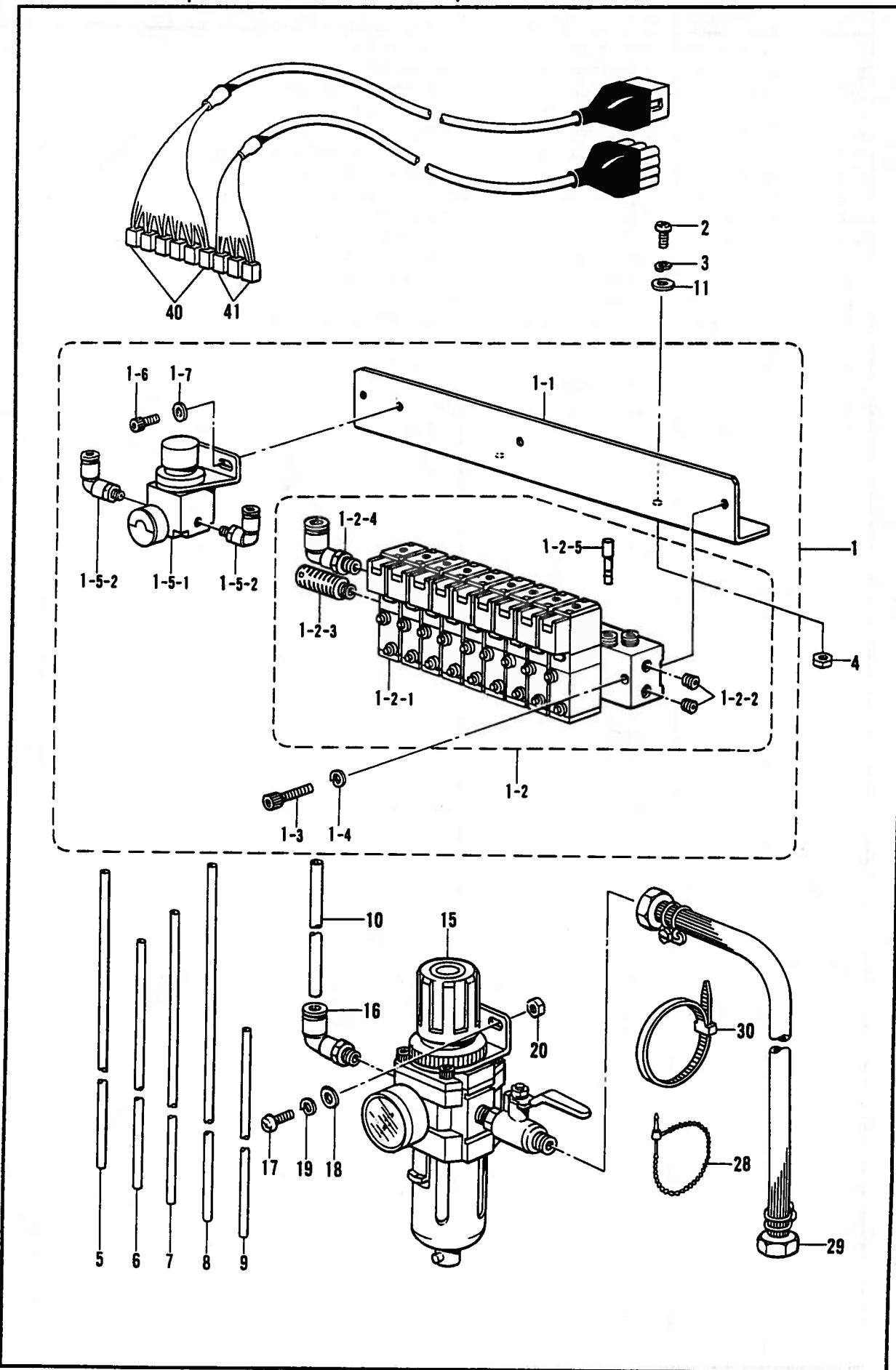
U. 空圧関係/Air pressure mechanism/Luftdruck/
