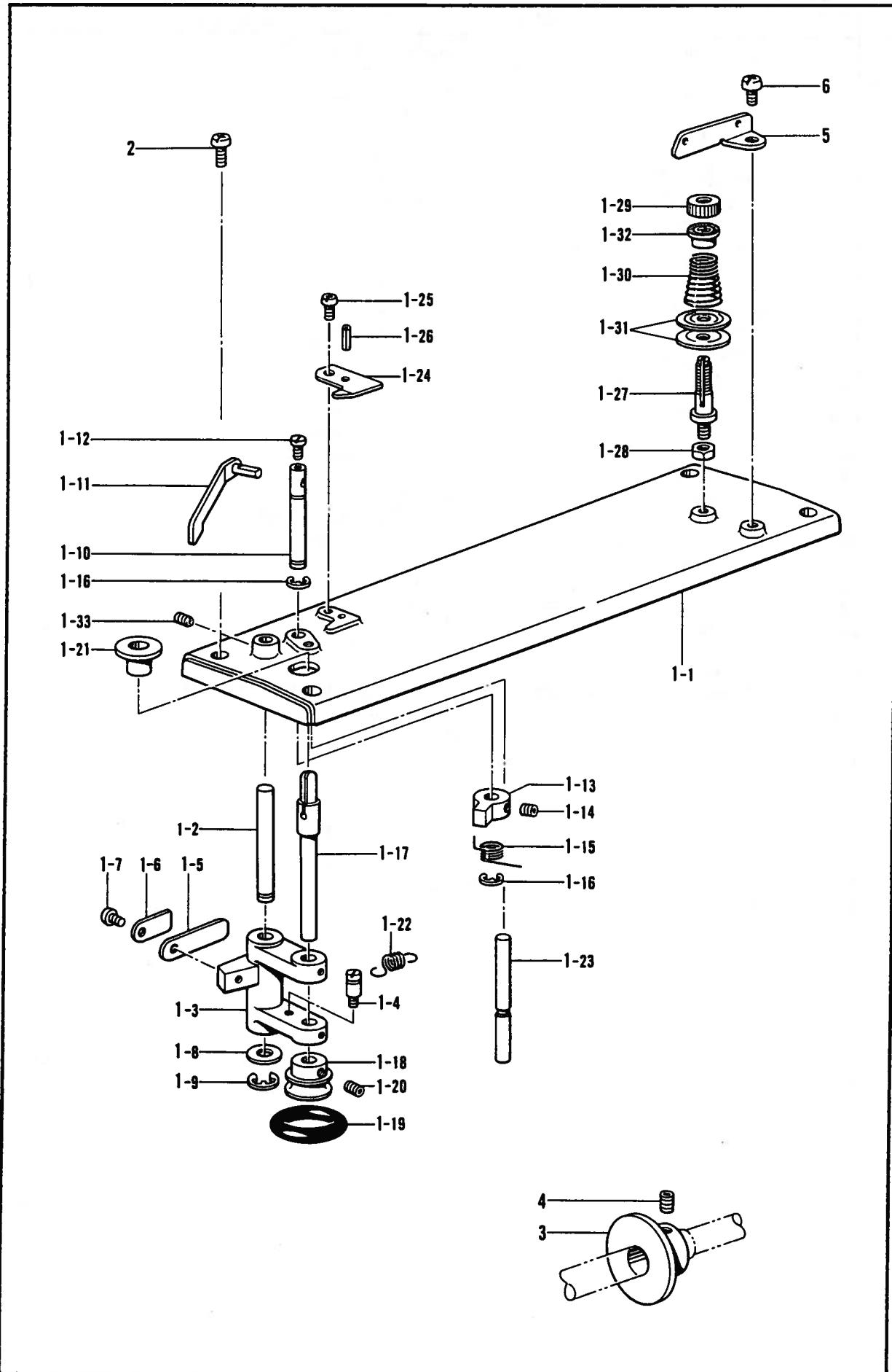
K. 糸巻関係 / Bobbin winder mechanism / Spuler/
