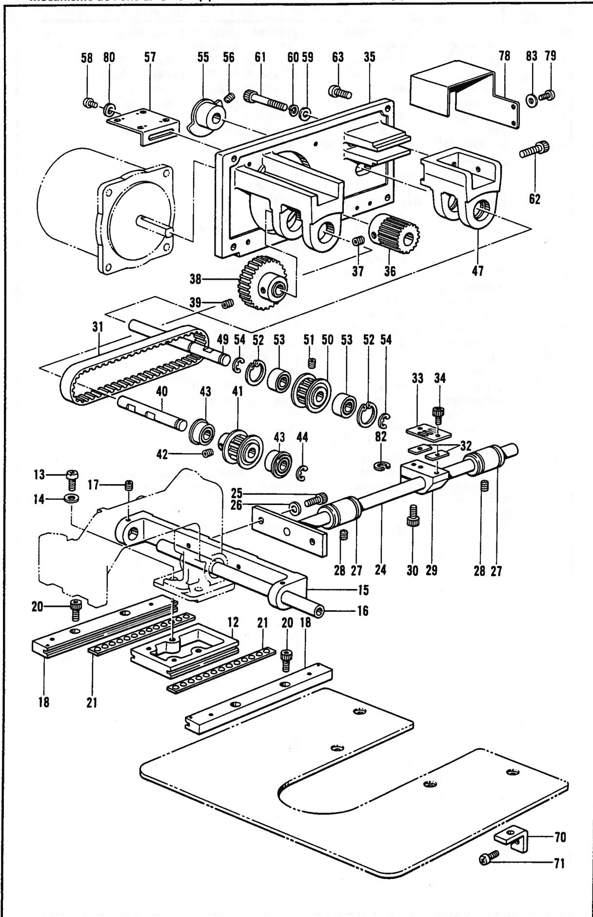
D2. 送り関係(1) /Feed mechanism (1)/Transportvorrichtung/
