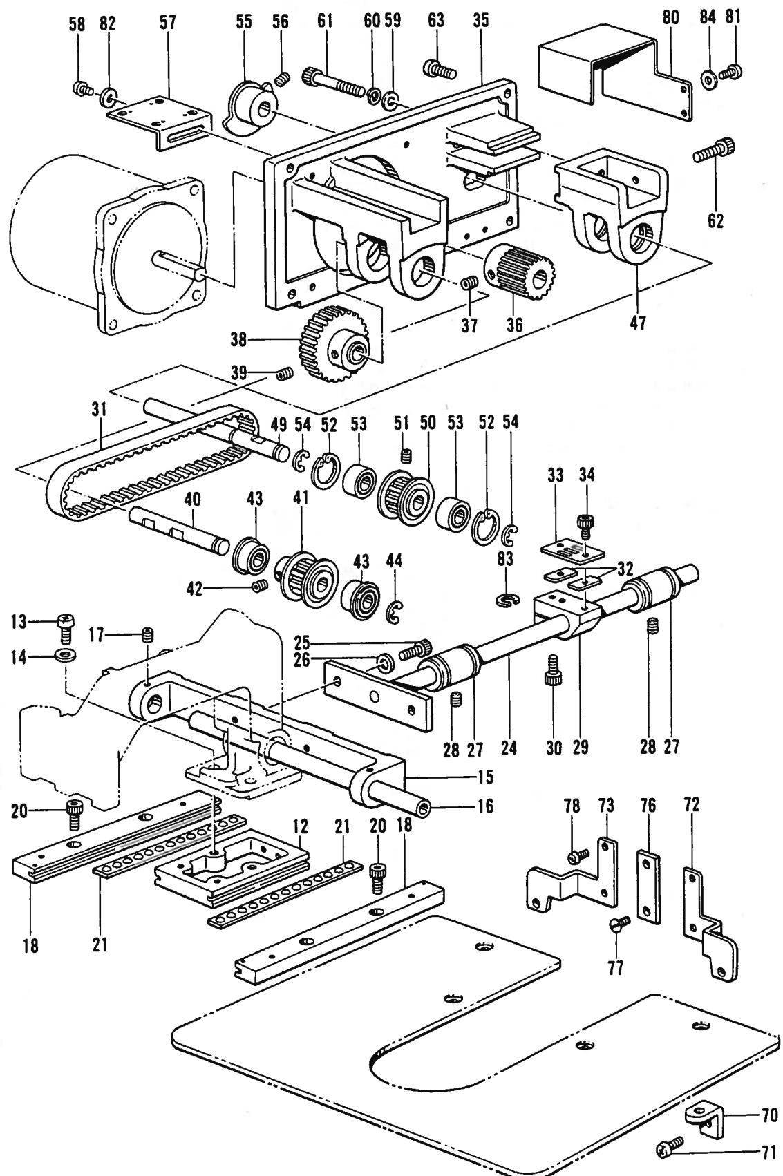
D2. 送り関係(1)/Feed mechanism (1)/Transportvorrichtung (1)/
