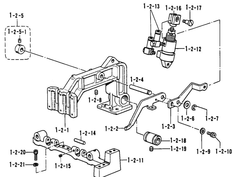
D1. 送り関係(1) /Feed mechanism (1)/Transportvorrichtung (1)/
