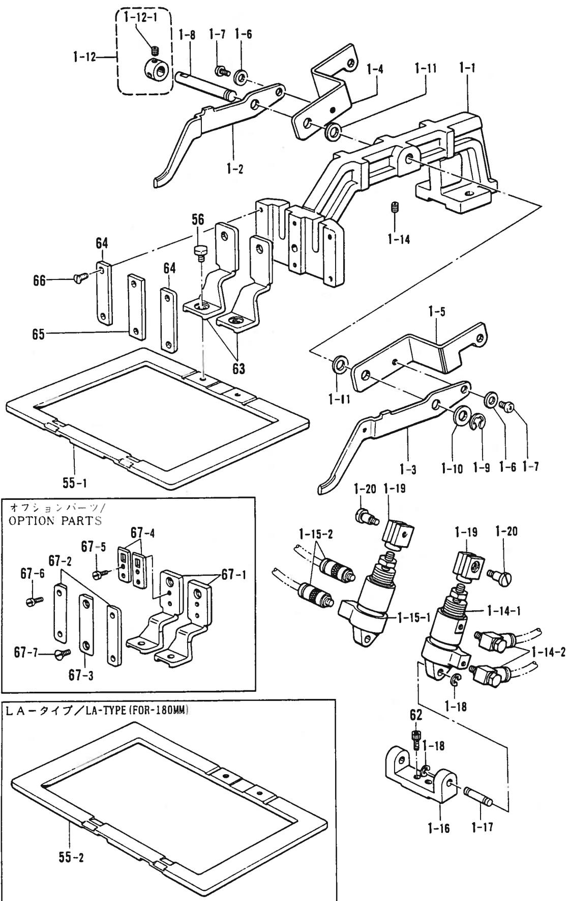
D1. 送り関係/Feed mechanism/Transportvorrichtung/
