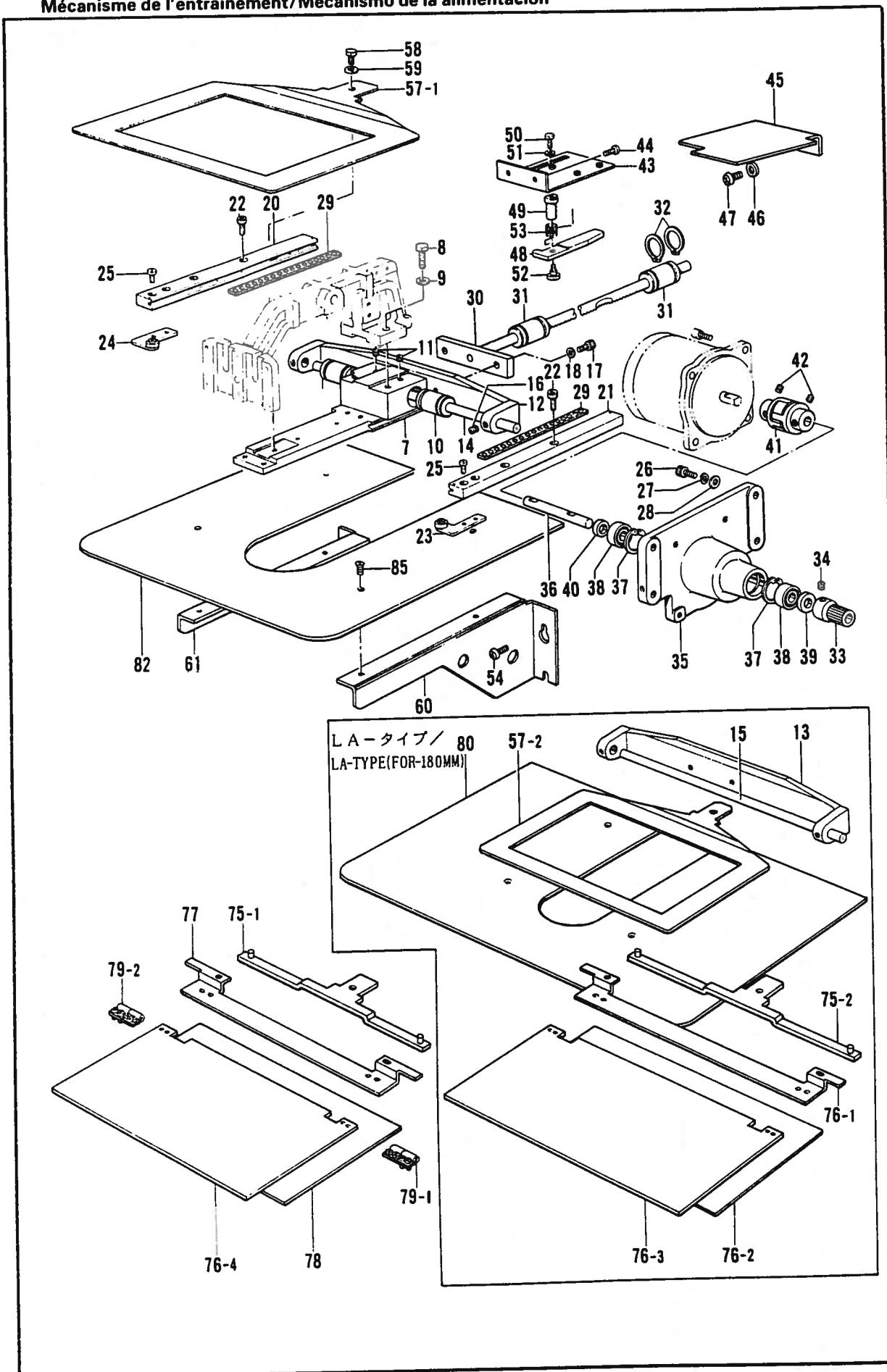
D2. 送り関係/Feed mechanism/Transportvorrichtung/
