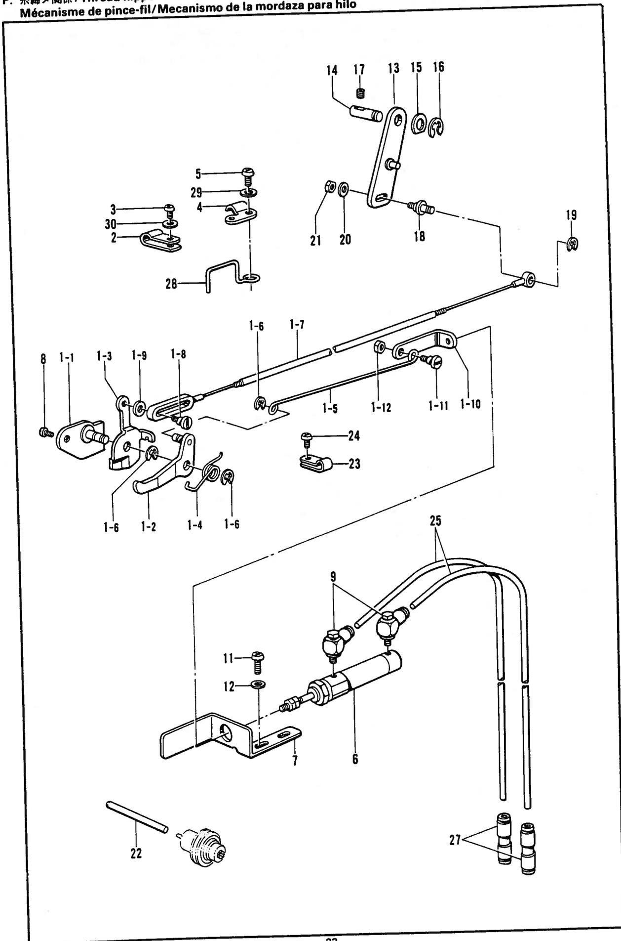
P. 糸締め関係/Thread nipper mechanism/Fadenspannvorrichtung/
