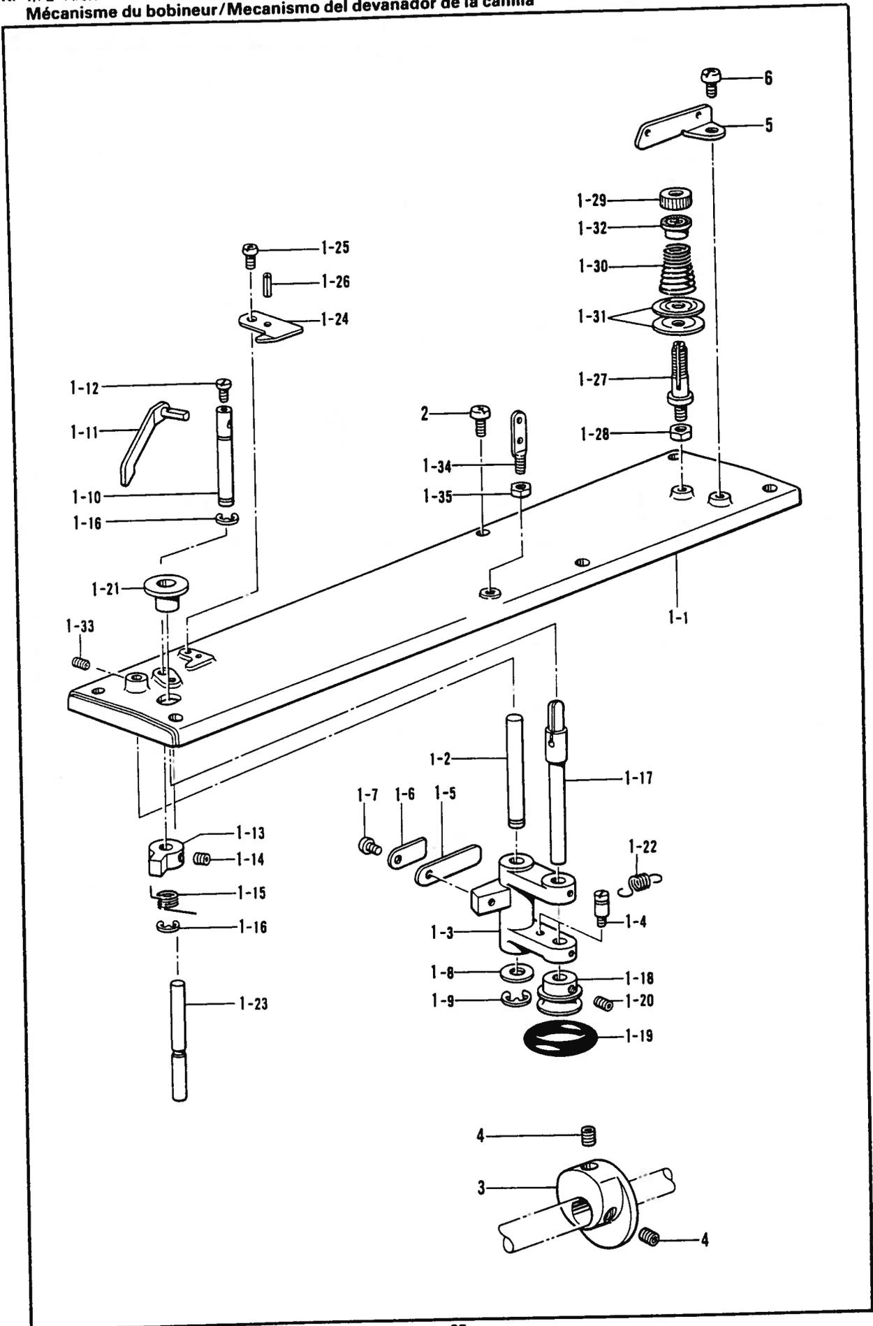
K. 糸巻キ関係/Bobbin winder mechanism/Spuler/
