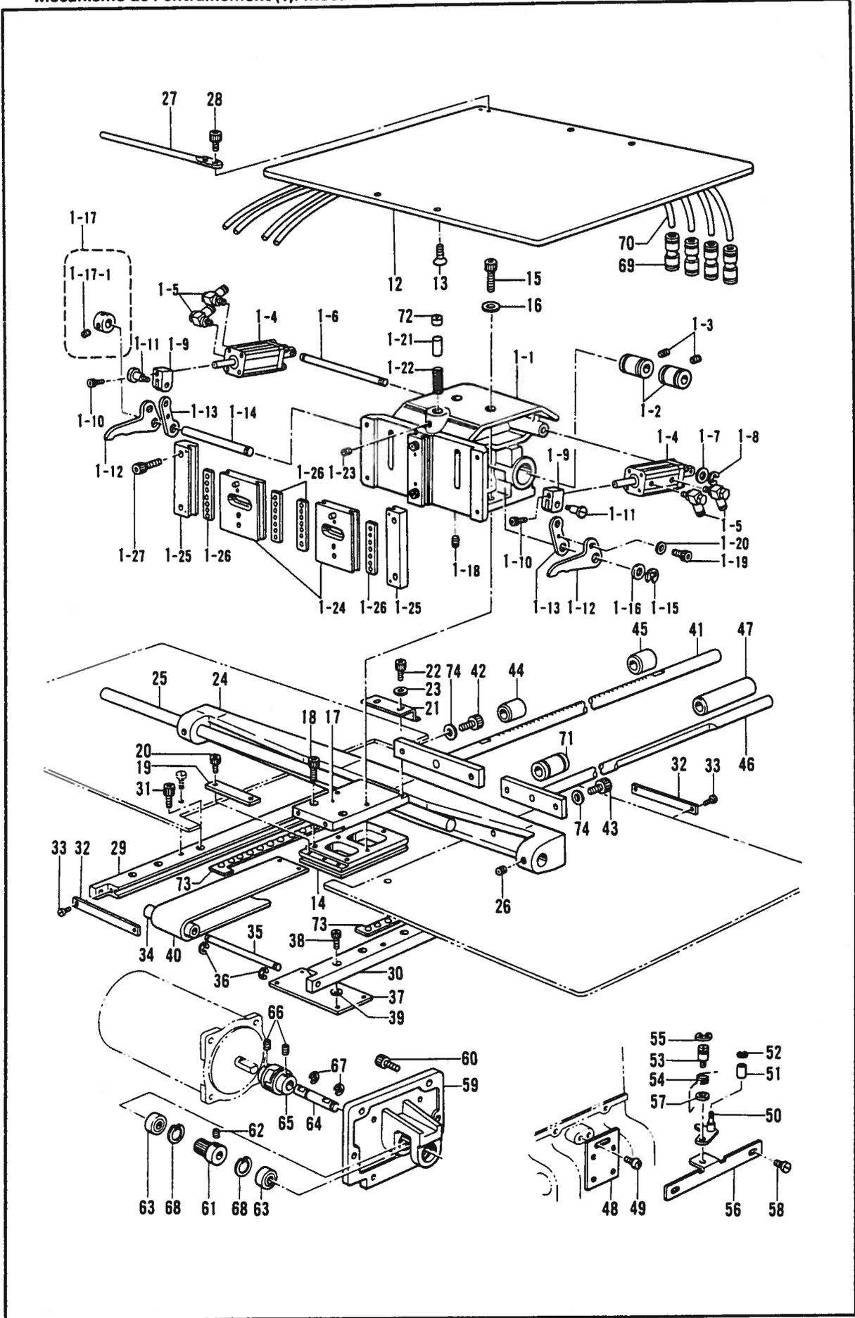
D1. 送り関係/Feed mechanism (1)/Transportvorrichtung (1)/
