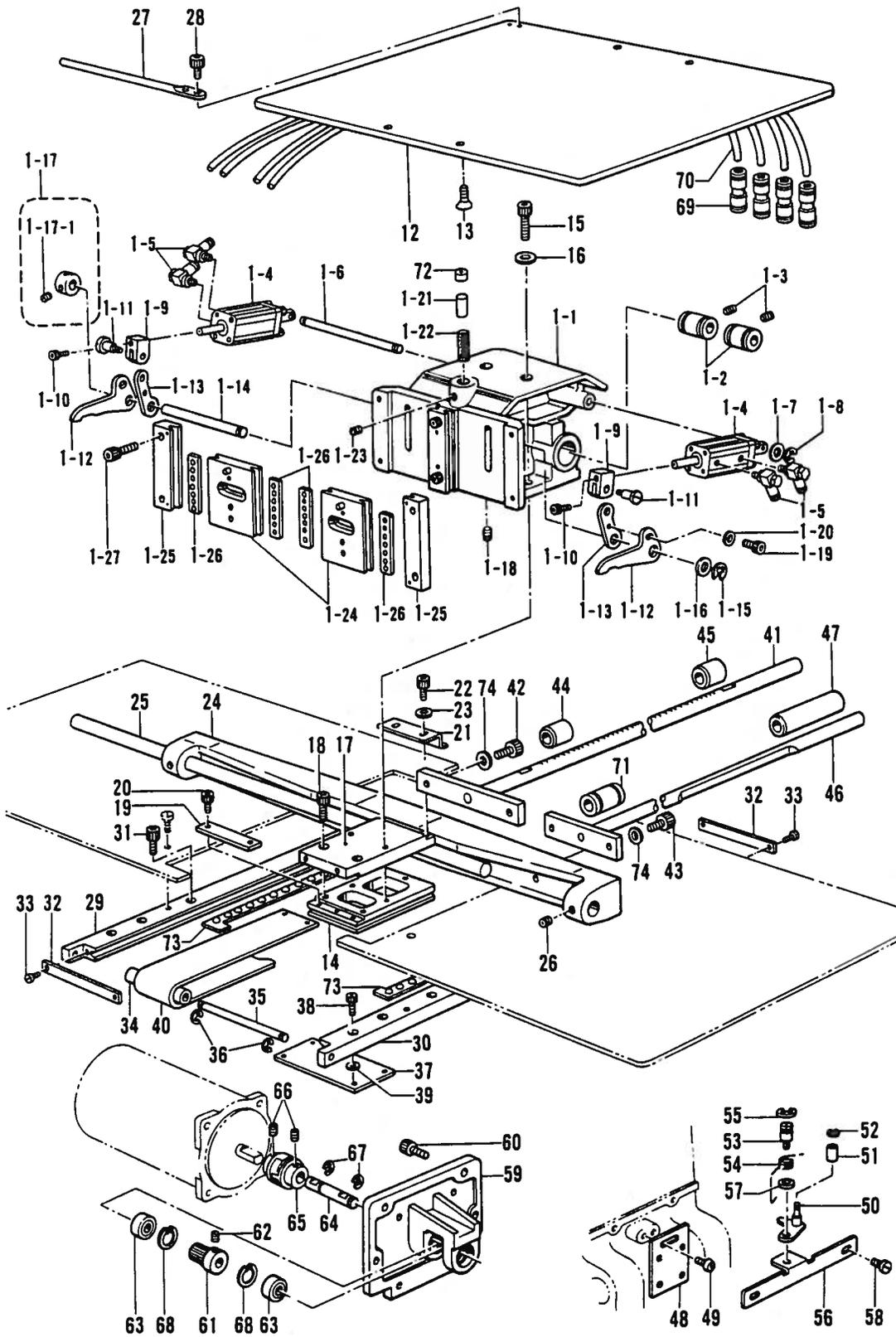
D1. 送り関係/Feed mechanism (1)/Transportvorrichtung (1)/
