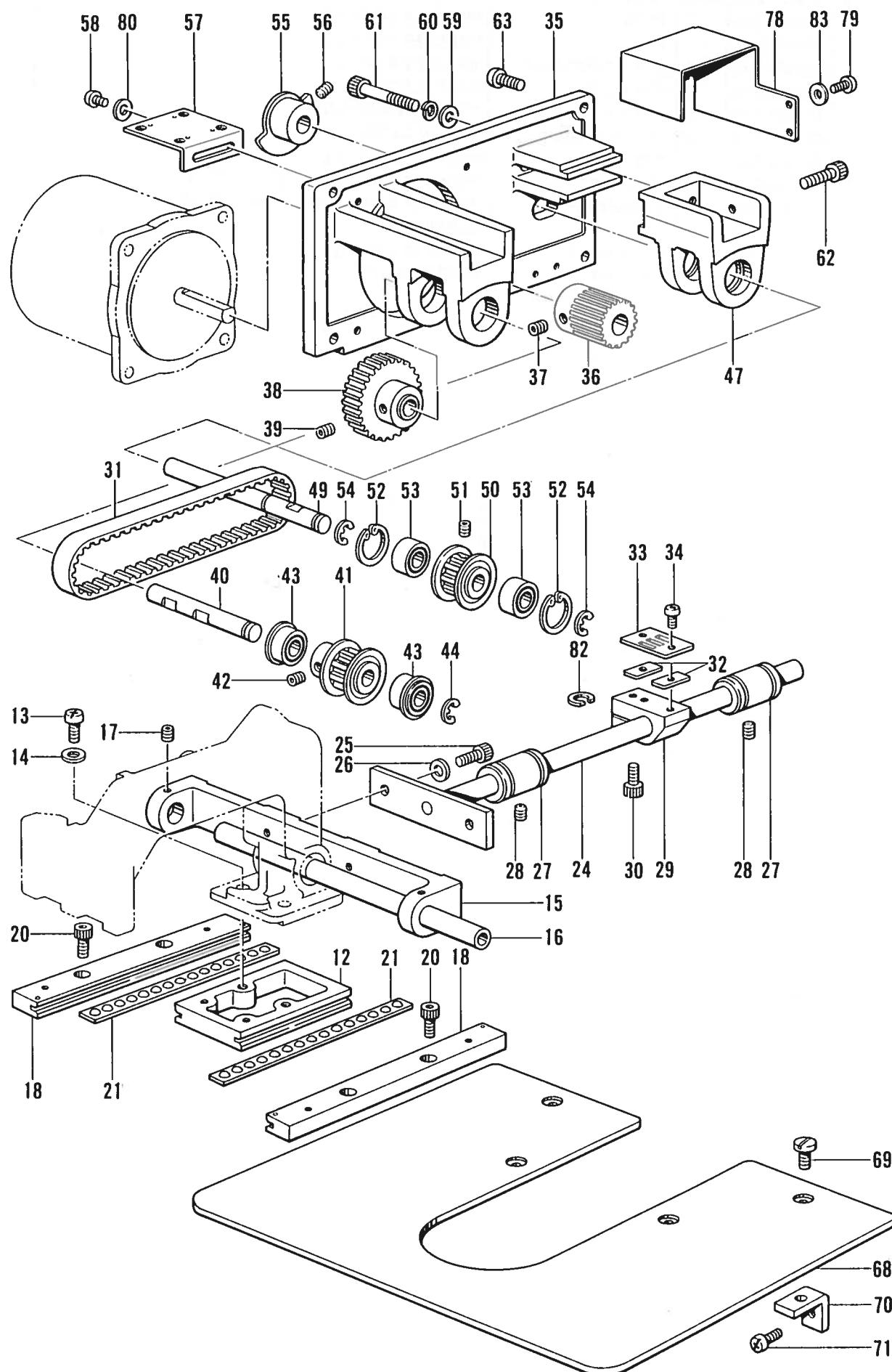
C. 送り関係 / Feed mechanism / Transportvorrichtung /
