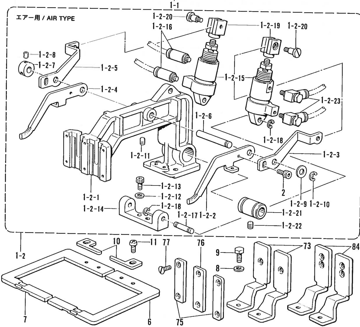
C. 送り関係 / Feed mechanism / Transportvorrichtung /
