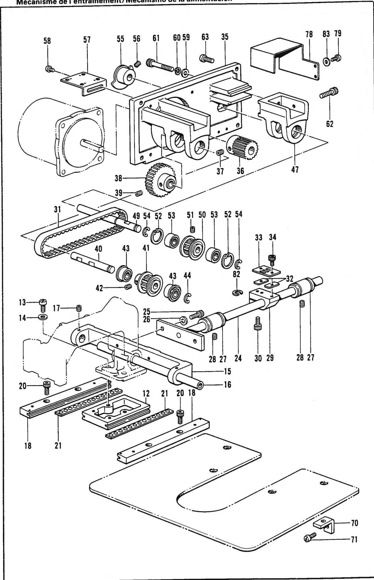
D3. 送り関係/Feed mechanism/Transportvorrichtung/
