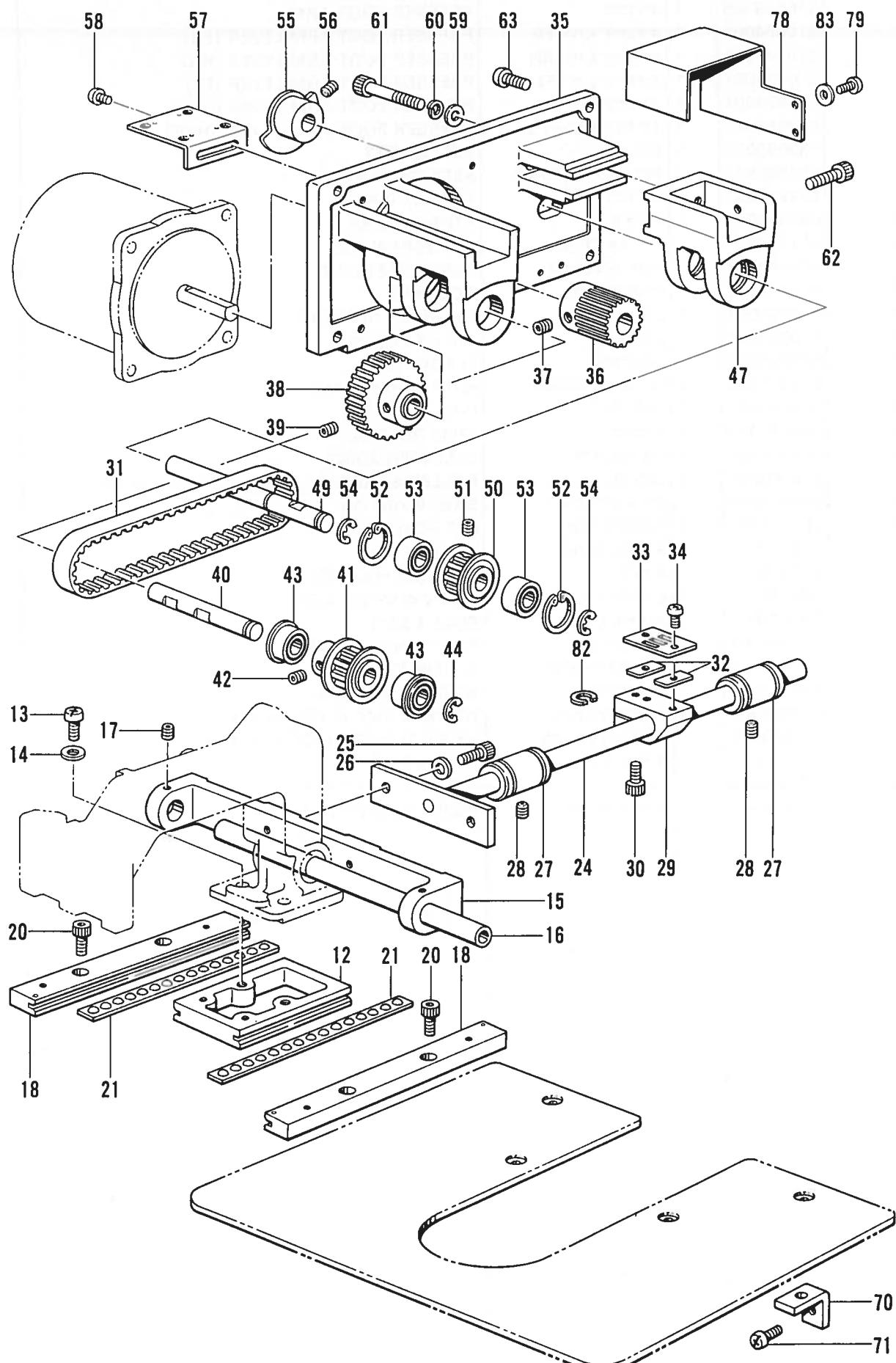
C. 送り関係(1) / Feed mechanism (1) / Transportvorrichtung (1) /
