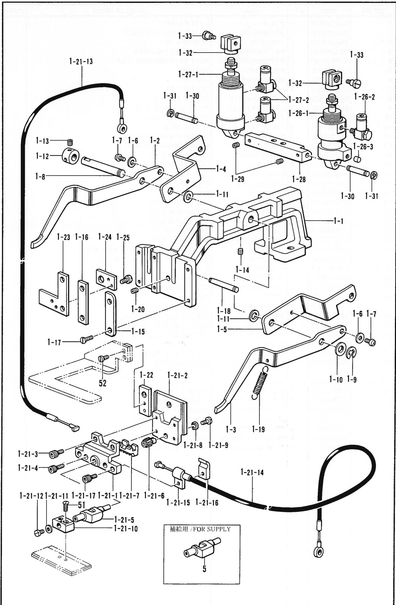
C. 送り関係/Feed mechanism/Transportvorrichtung/
