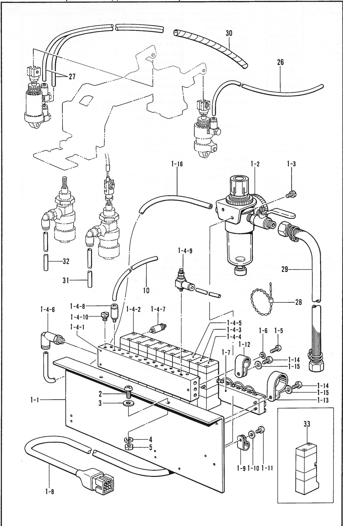
T. 空圧関係(2)/Air pressure mechanism (2)/Luftdruck (2)/
