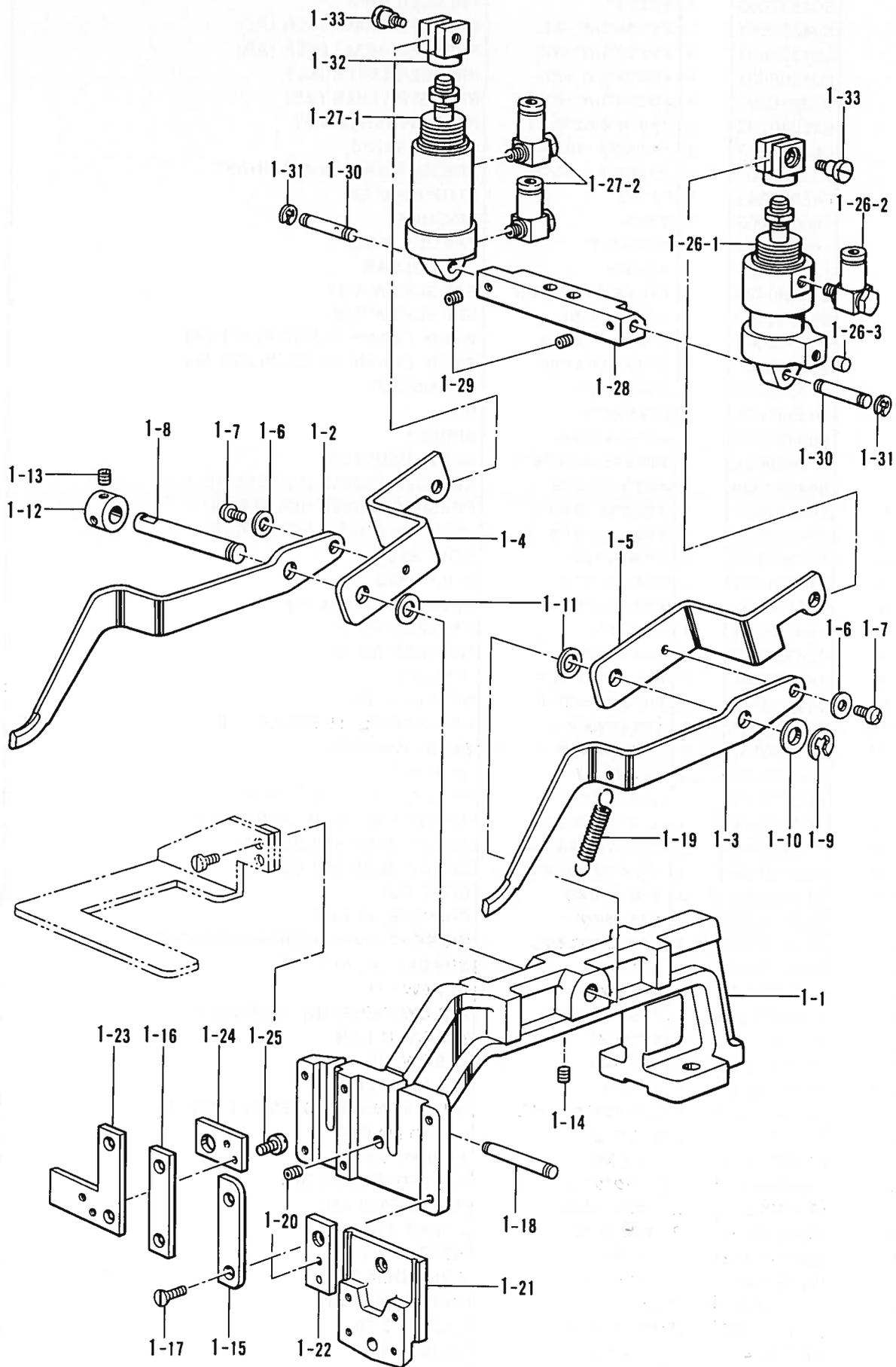
C. 送り関係/Feed mechanism/Transportvorrichtung/
