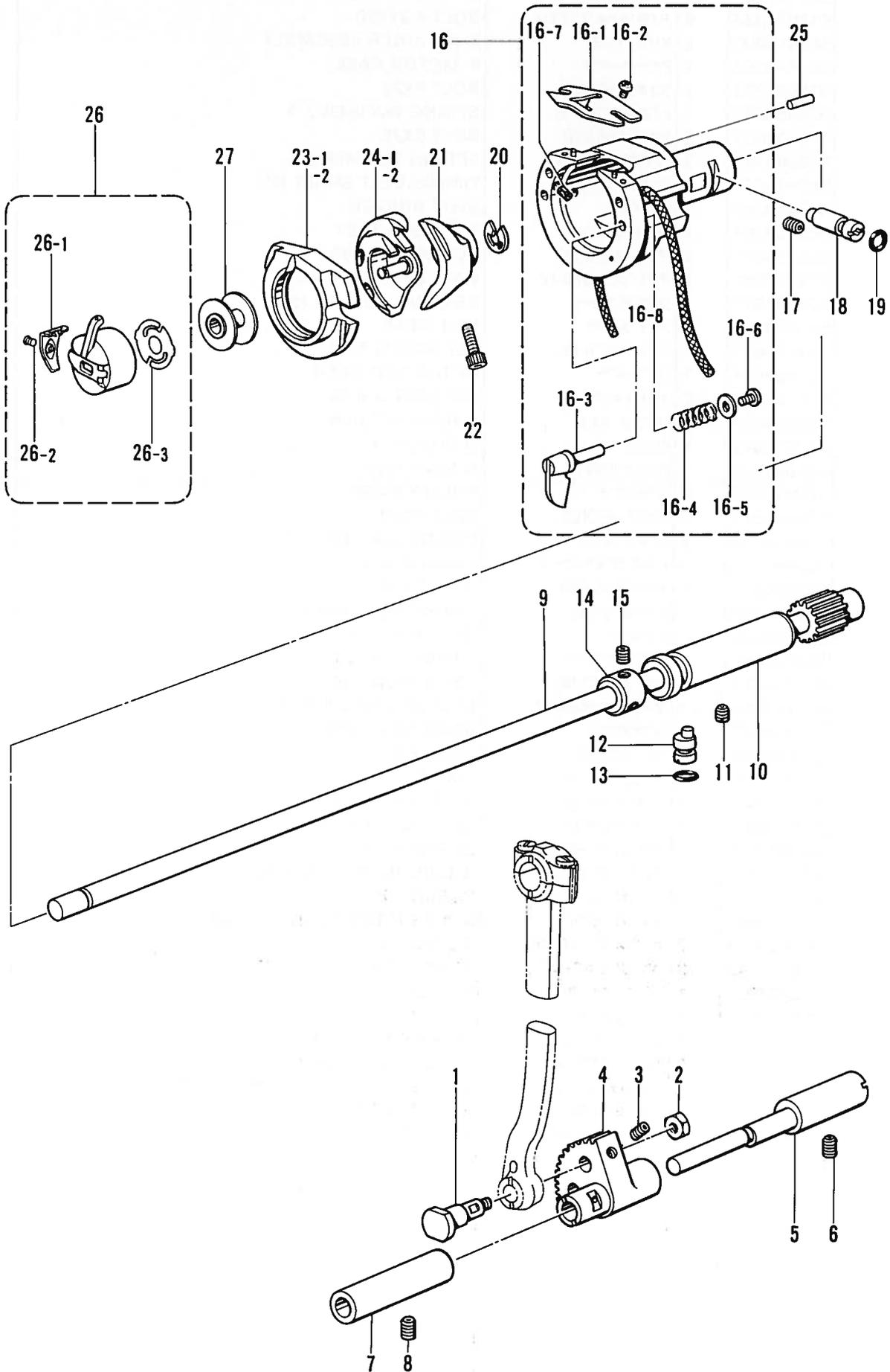
F. 下軸関係/Lower shaft mechanism/Untere Welle/
