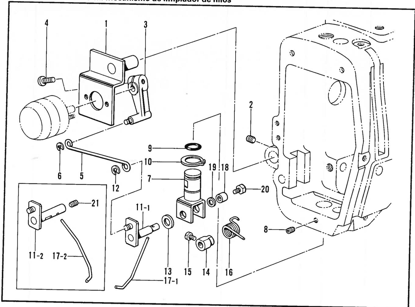
K. 糸巻関係/Bobbin winder mechanism/Spuler/
