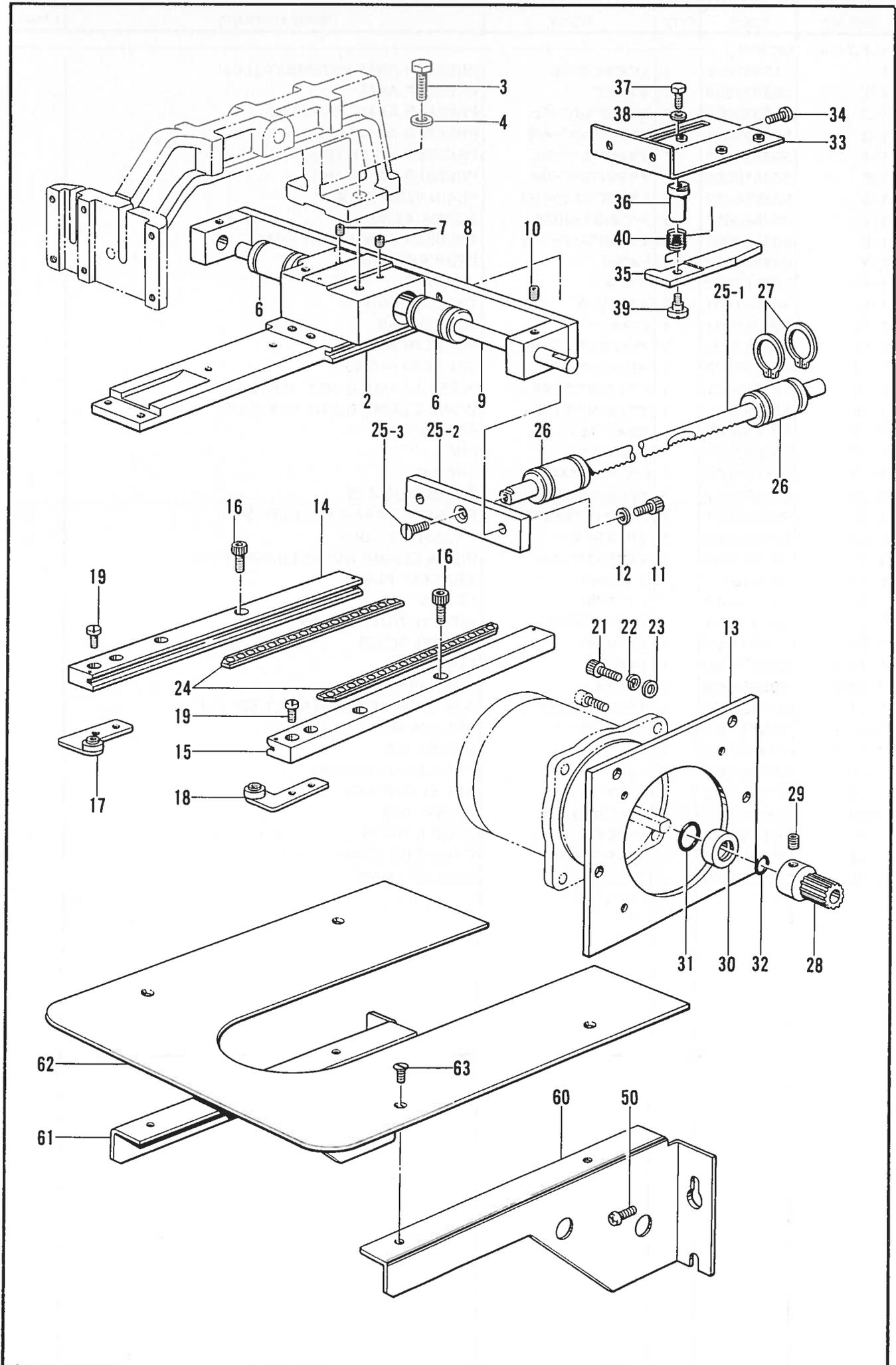
C. 送り関係/Feed mechanism/Transportvorrichtung/
