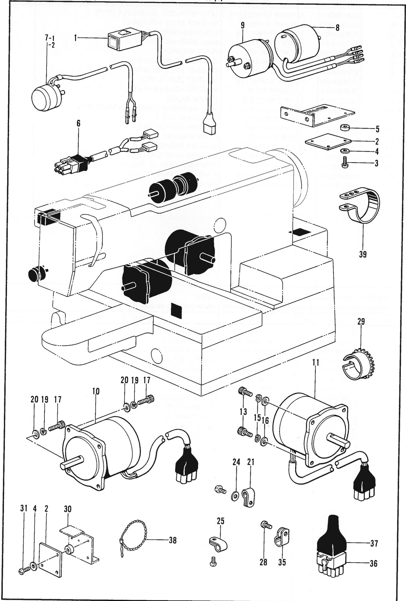
P. 電装品関係(1)/Power supply equipment mechanism (1)/Stromversorgung (1)/
