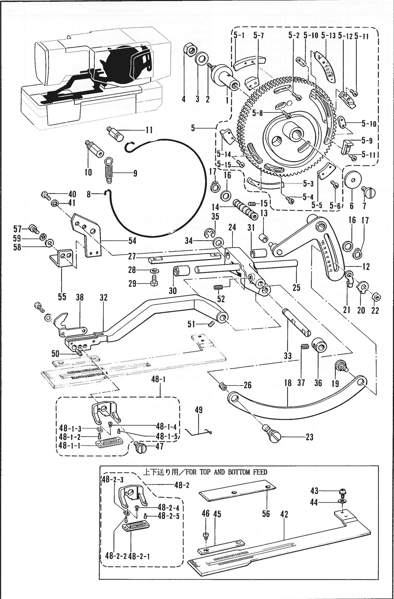
J. 送り関係/Feed mechanism/Transportvorrichtung/
