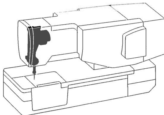
B. 針棒関係/Needle bar mechanism/Nadelstangenvorrichtung/
