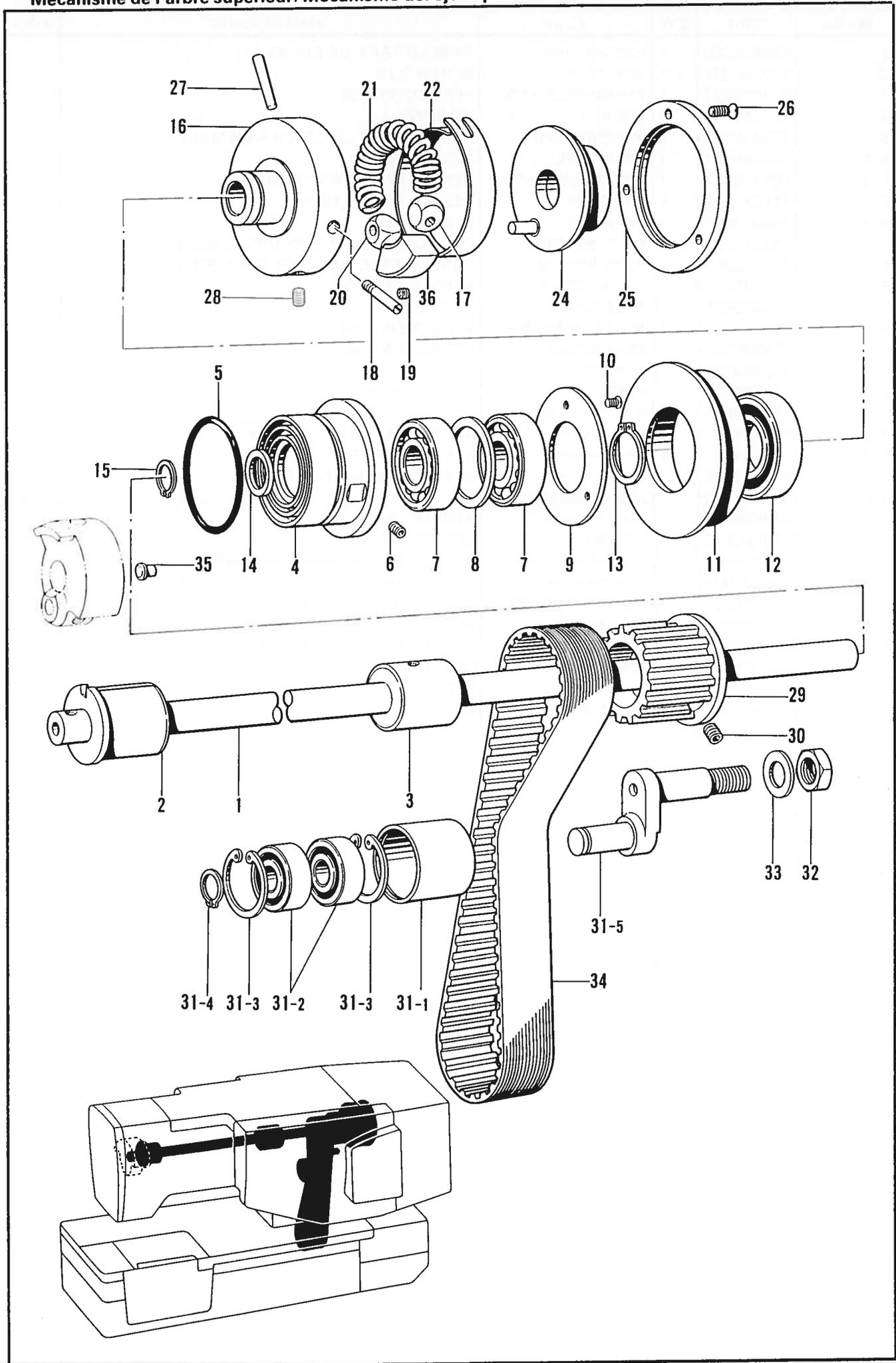
C. 上軸関係 / Upper shaft mechanism / Obere Welle /
