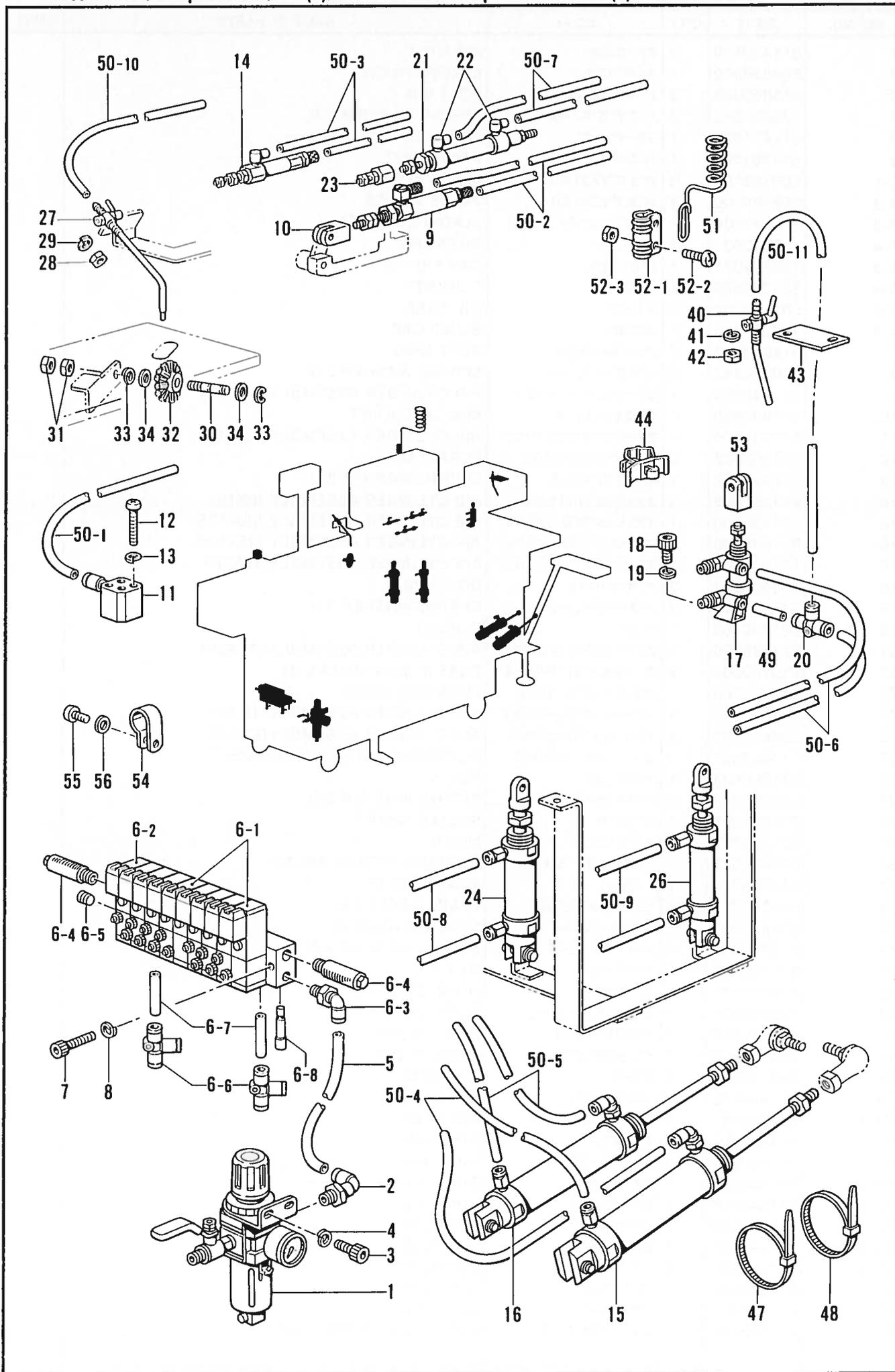
C1. 空圧関係(1)/Air pressure mechanism (1)/Luftdruck (1)/
