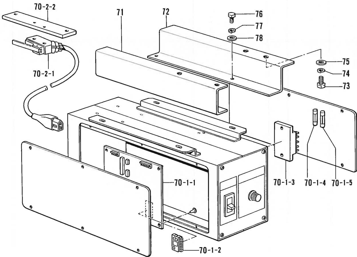
D1. 電装品関係(2)/Power supply equipment mechanism (2)/Stromversorgung (2)/
