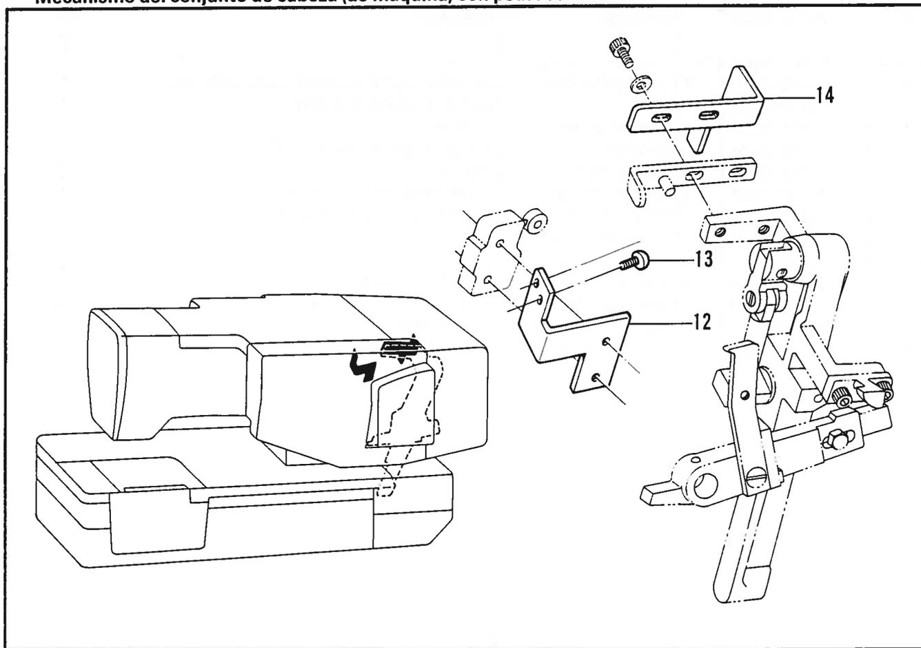
P. 下軸関係 / Lower shaft mechanism / Untere Welle /
