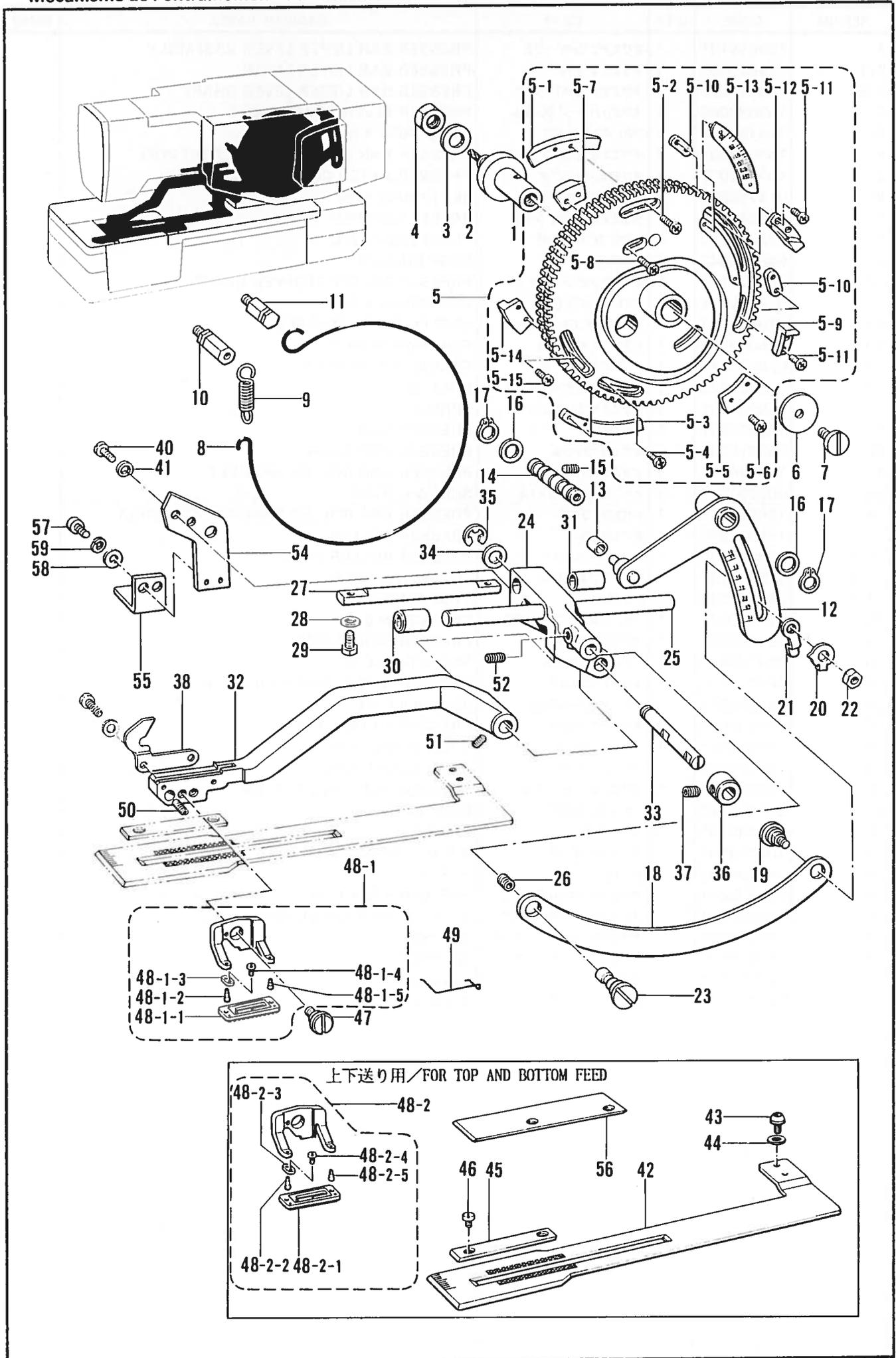
J. 送り関係/Feed mechanism/Transportvorrichtung/
