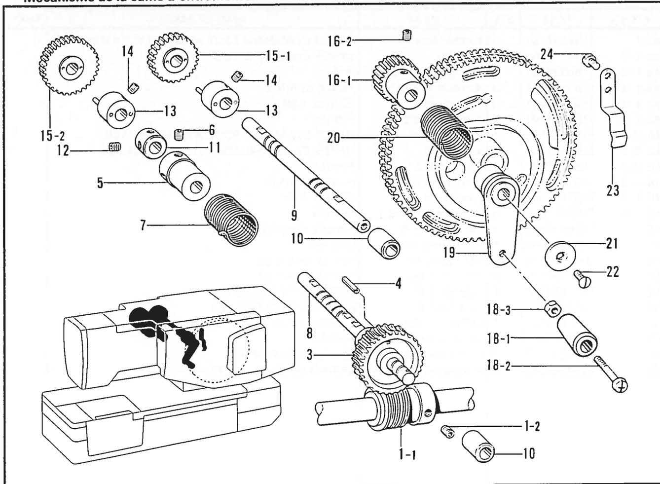
L. 糸切れ感知関係 / Thread breakage detector mechanism / Fadenbruchfühler /
