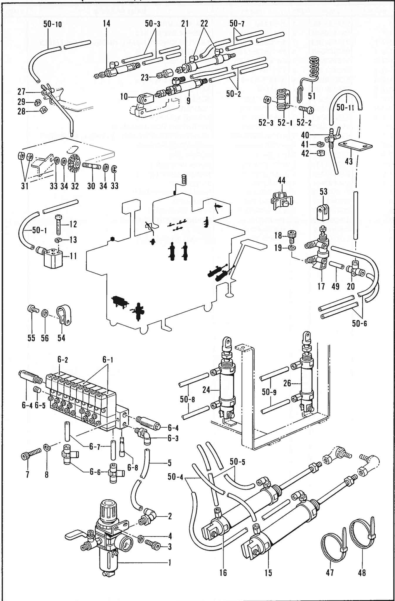
C1. 空圧関係(1)/Air pressure mechanism (1)/Luftdruck (1)/
