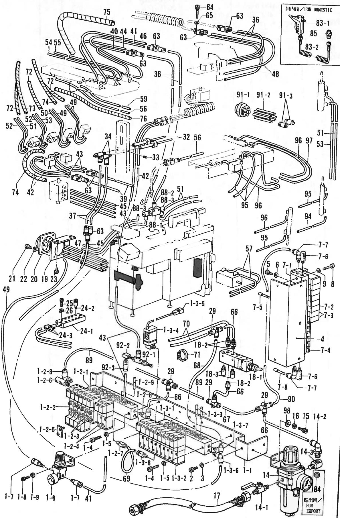
X. 空圧関係/Air pressure mechanism/Luftdruck/
