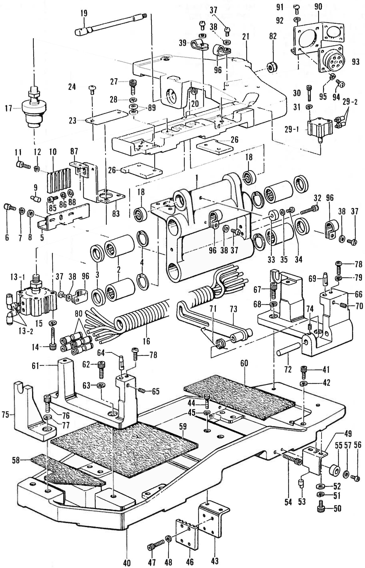
Q. 駆動側・送り関係/Drive, feed mechanism/Transporvorrichtung/
