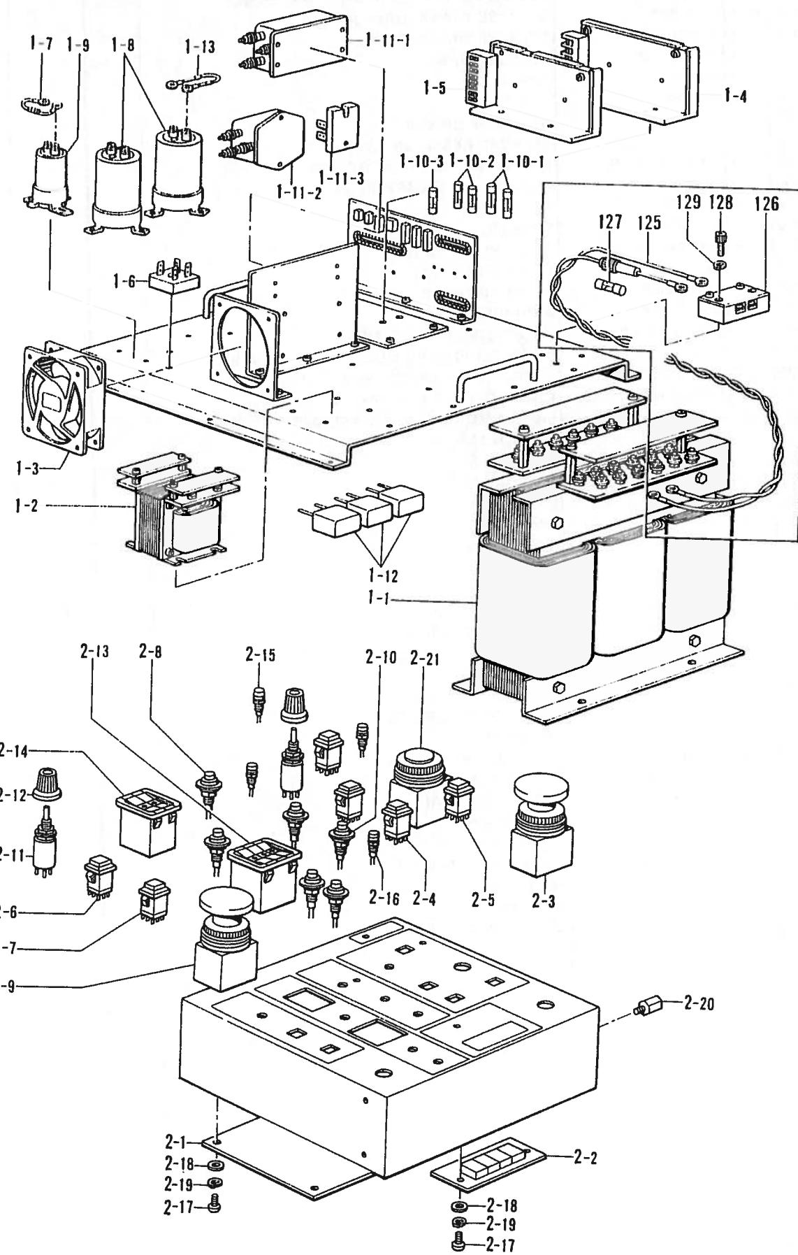
V. 電装品関係(2)/Power supply equipment mechanism (2)/Stromversorgung (2)/
