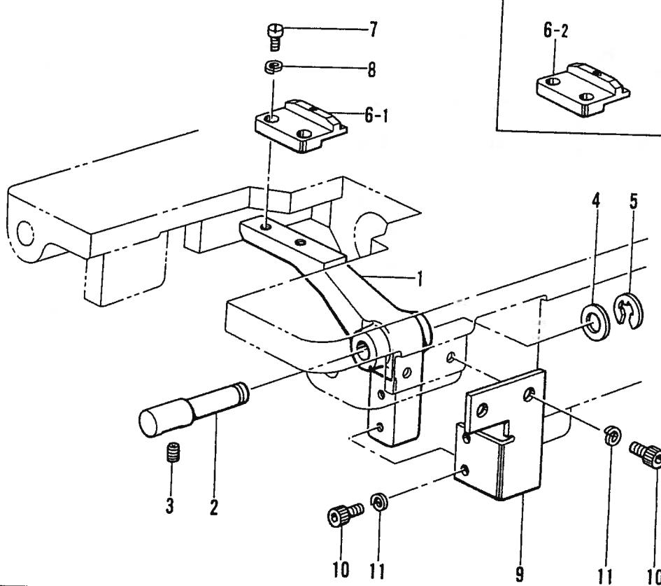
D. 糸切れ感知関係 / Thread breakage detector mechanism / Fadenbruchfühler /
