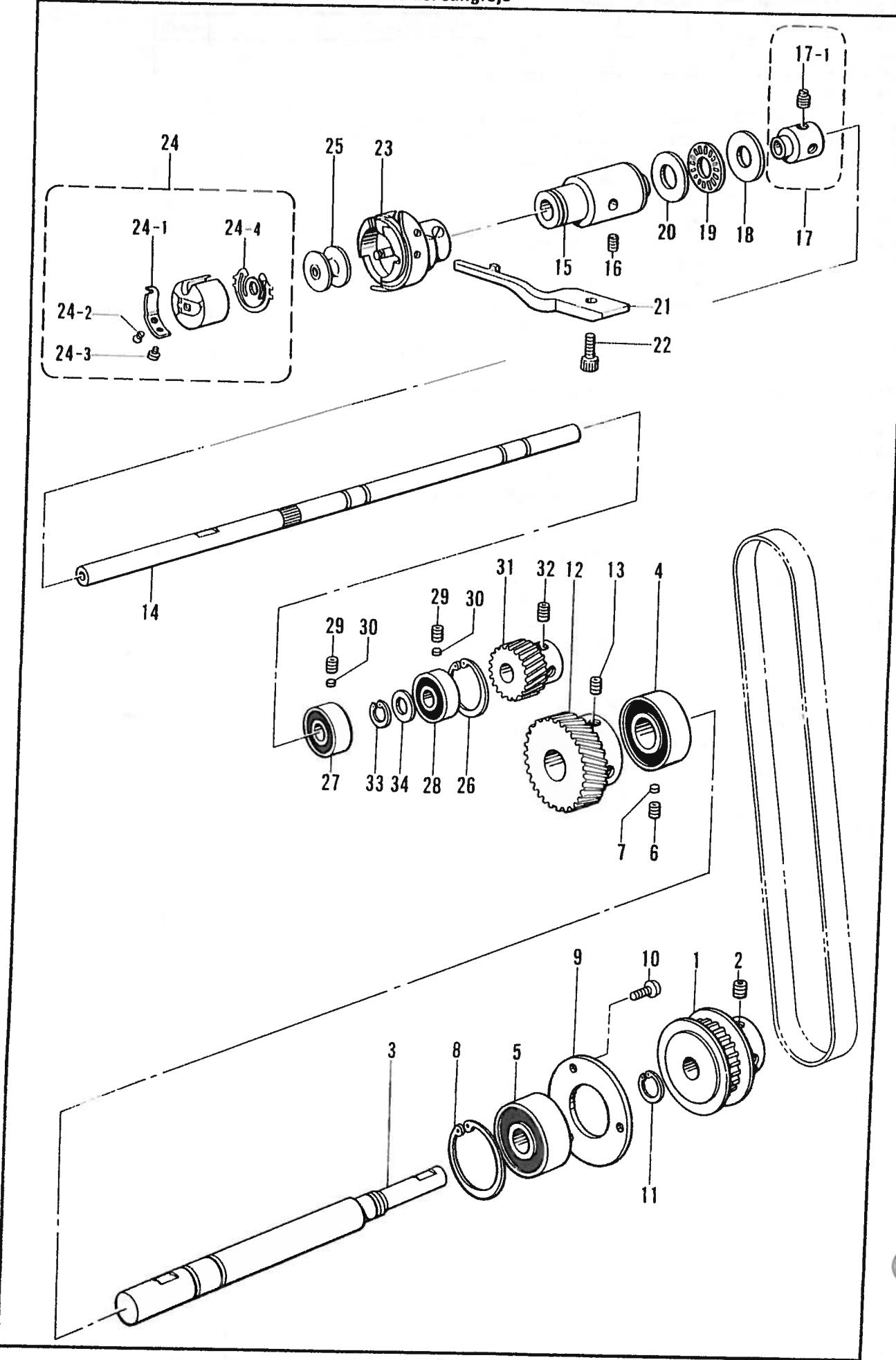
F. カマ関係/Rotary hook mechanism/Greifervorrichtung/
