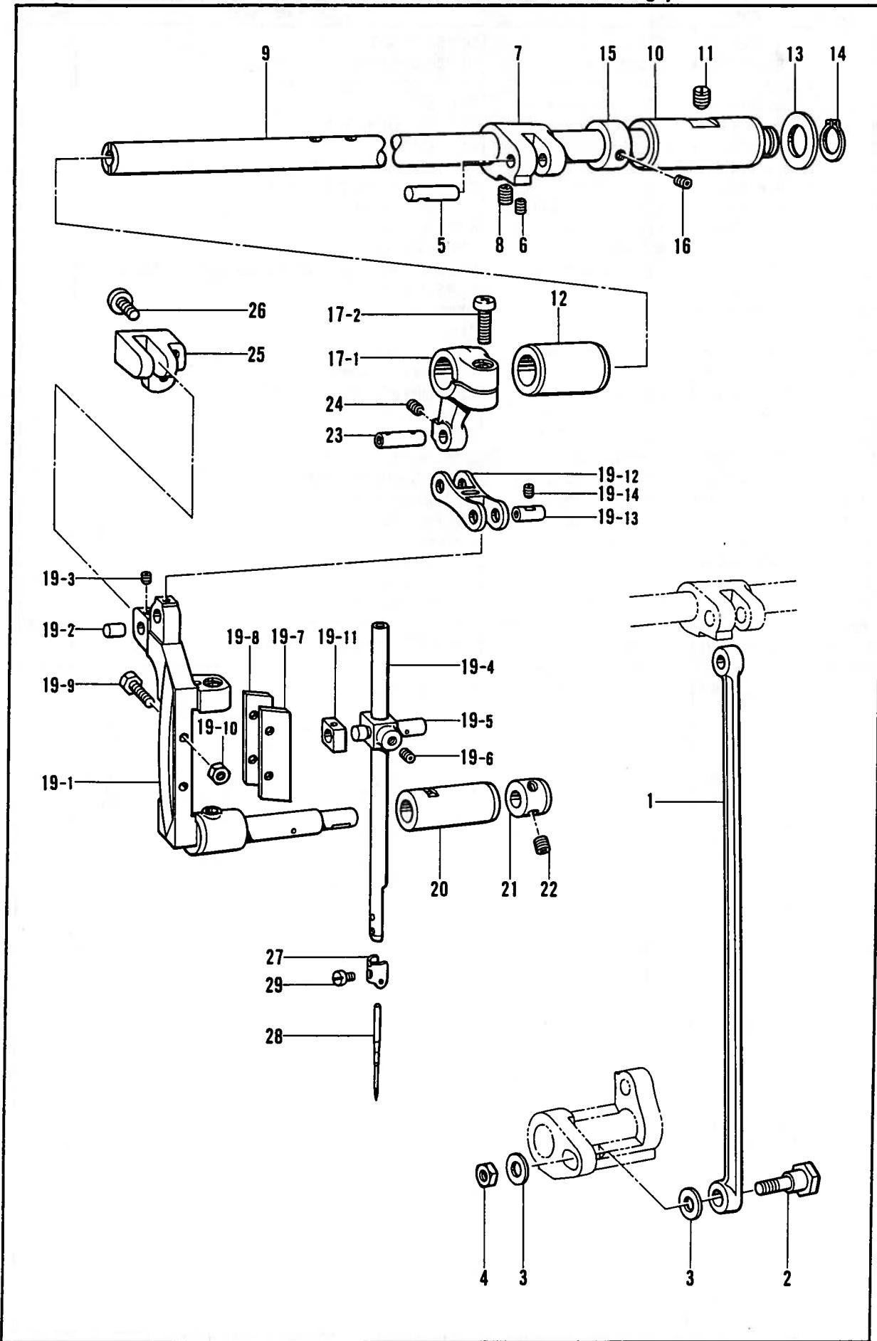
D. 針送り関係 / Needle feed mechanism / Nadelstange transportvorrichtung /
