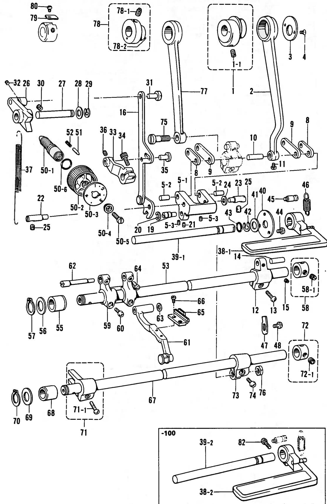
E. 送り関係/Feed mechanism/Transportvorrichtung/
