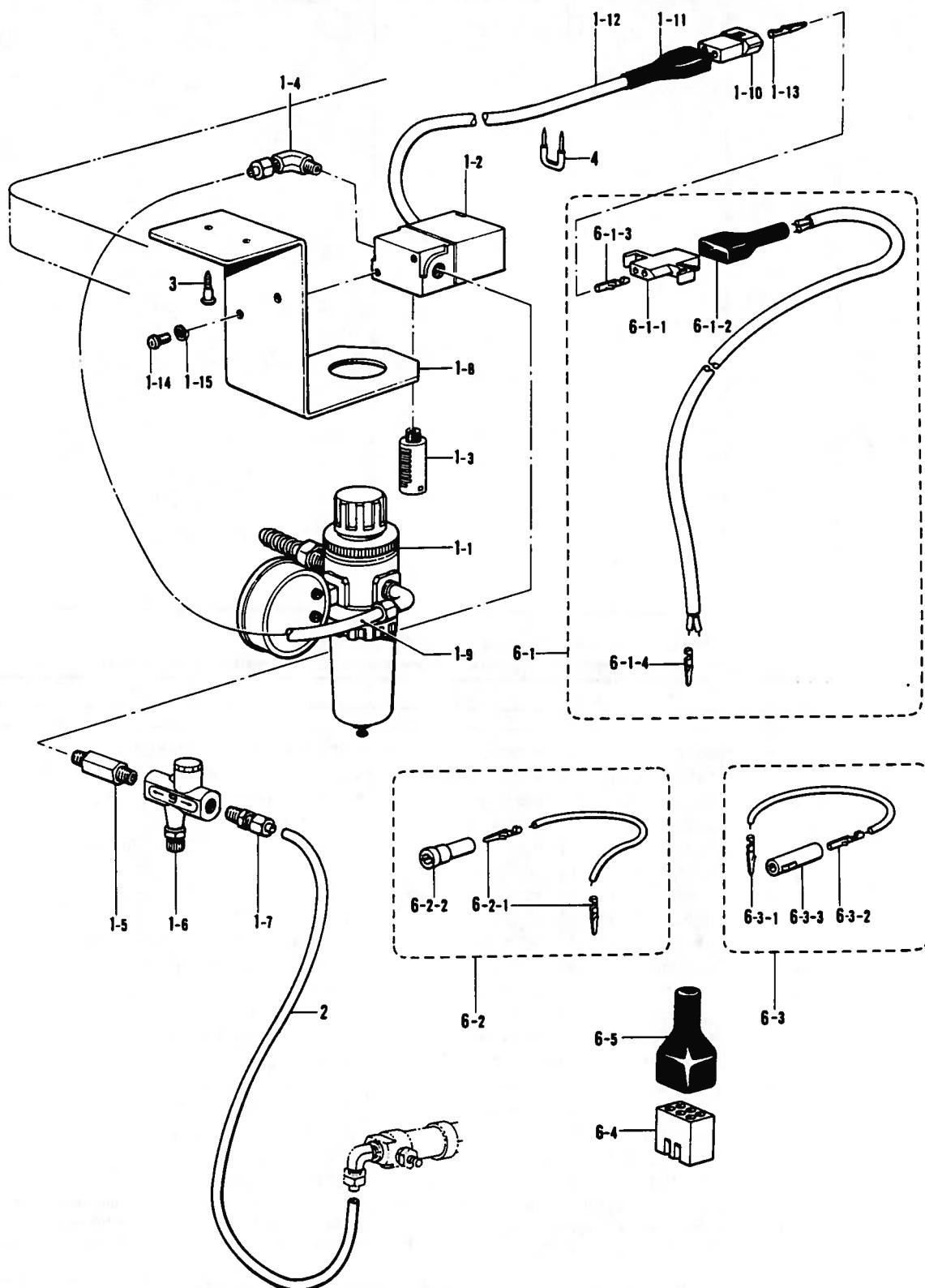
T. 空圧関係/Air pressure mechanism/Luftdruck/
