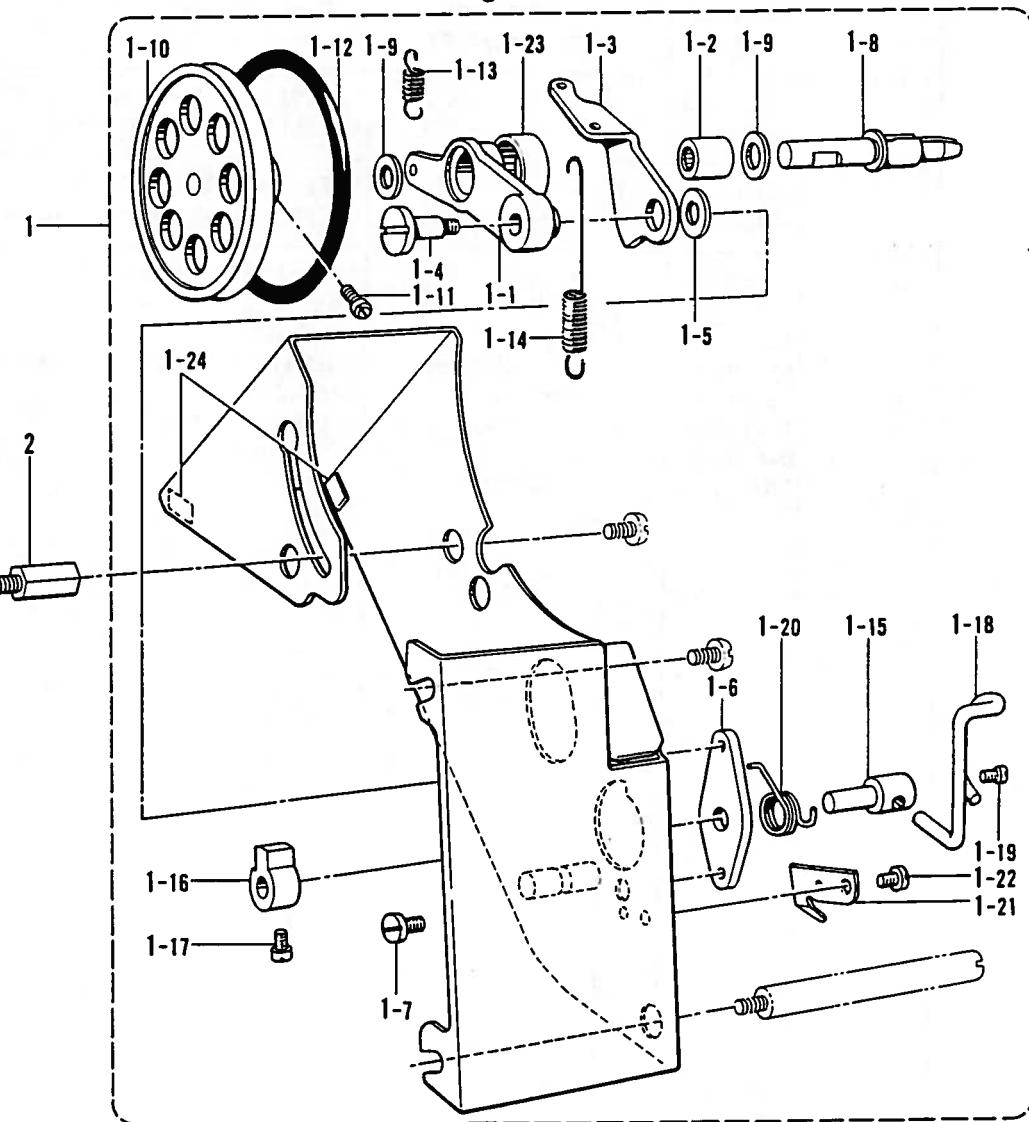
X. 糸巻き関係 / Bobbin winder mechanism / Spuler /
