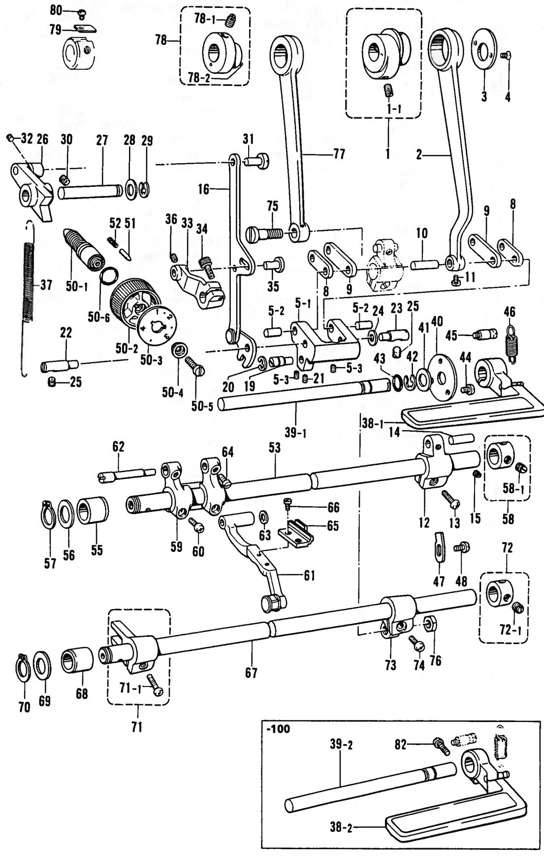
E. 送り関係/Feed mechanism/Transportvorrichtung/
