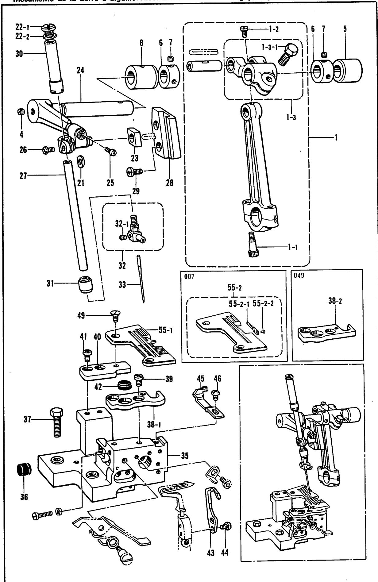
D. 針棒関係/Needle bar mechanism/Nadelstangenvorrichtung/
