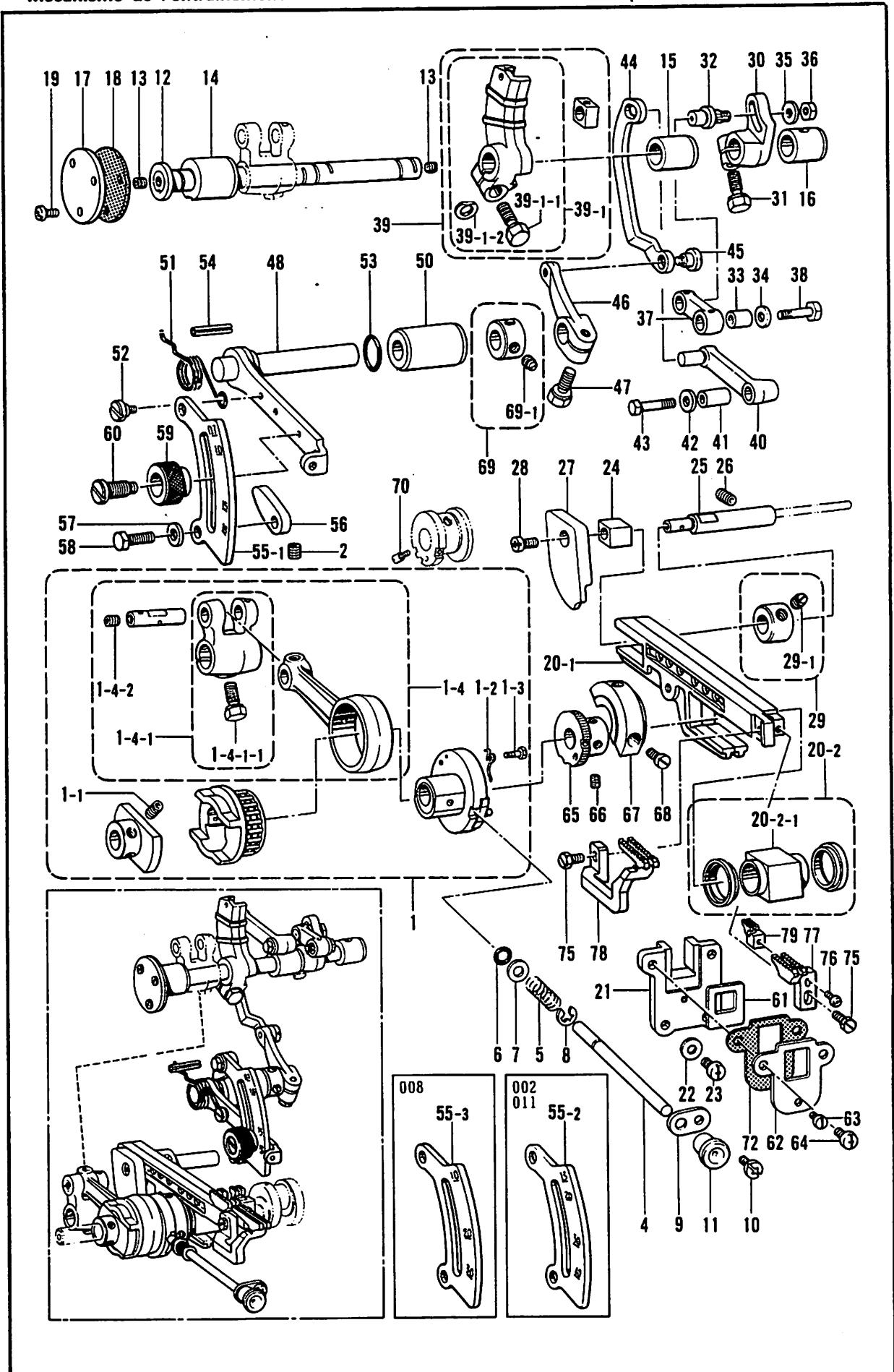
F. 送り関係/Feed mechanism/Transportvorrichtung/
