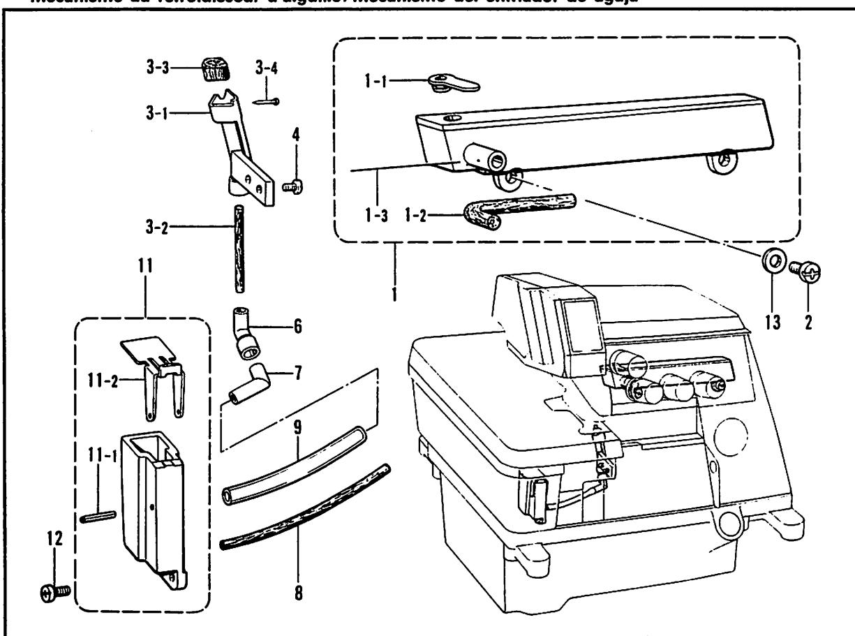
B. 駆動軸関係/Crank shaft mechanism/Kurbelwelle/
