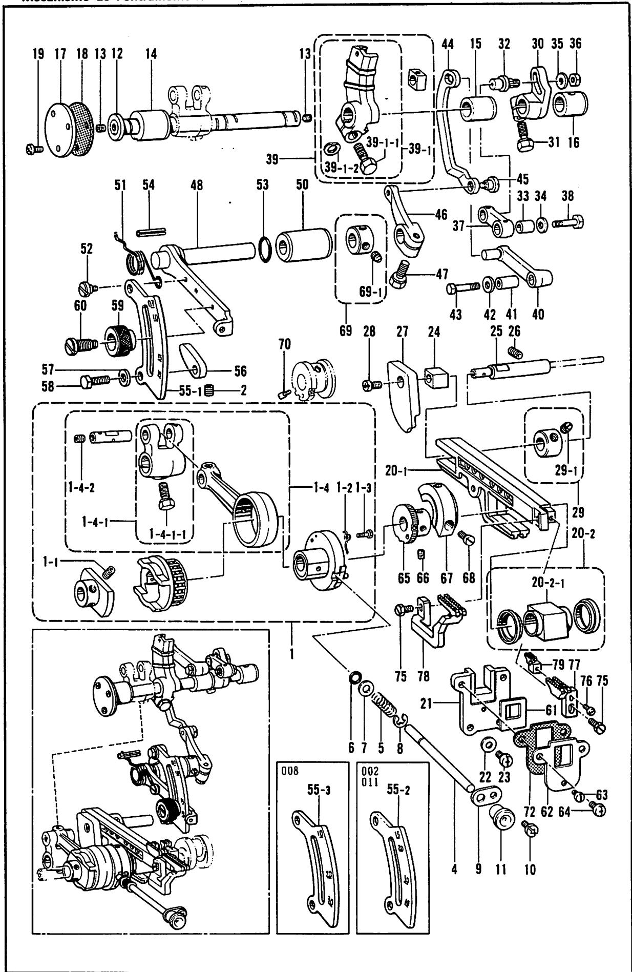
F. 送り関係/Feed mechanism/Transportvorrichtung/
