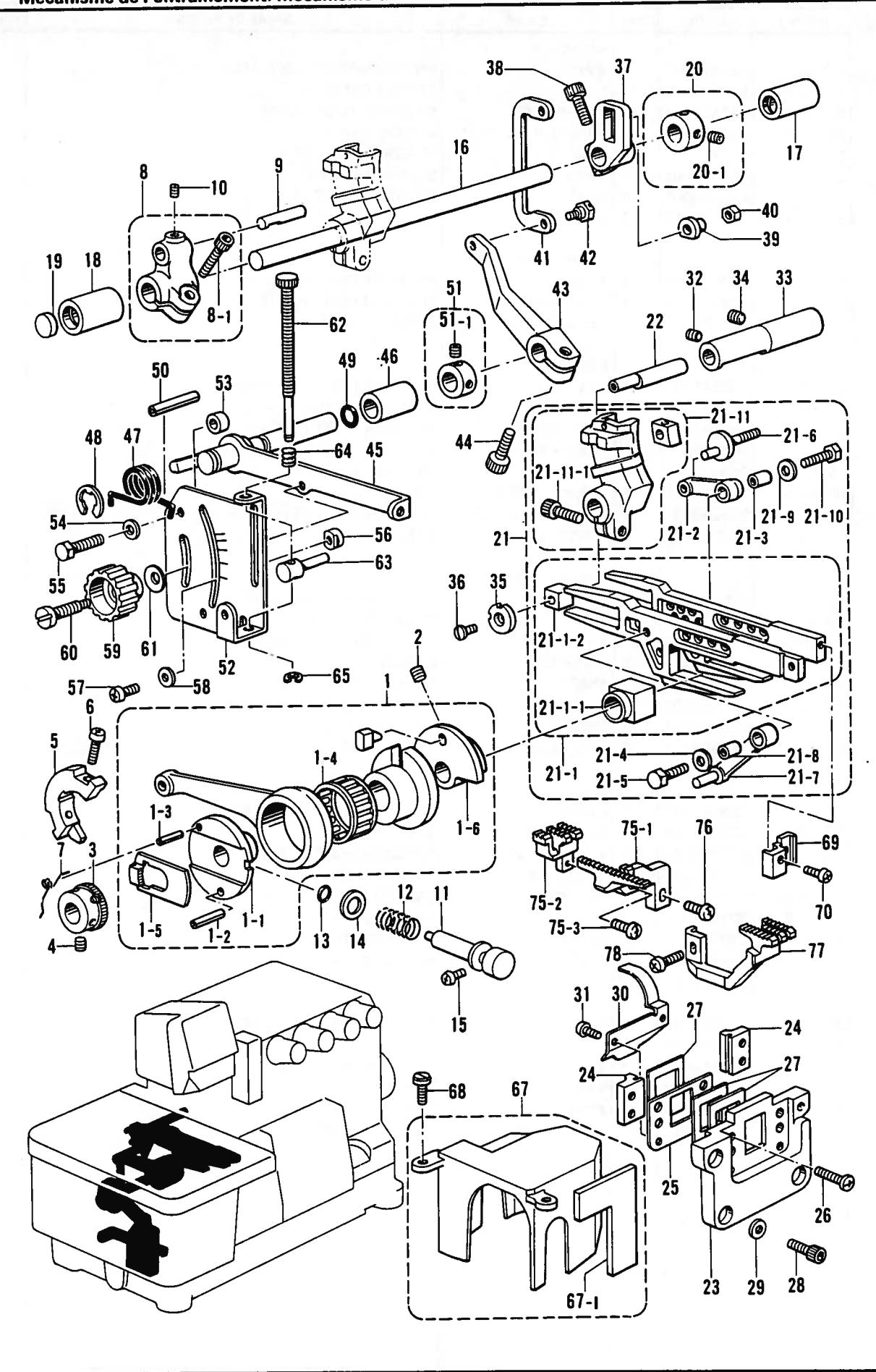
E. 送り関係/Feed mechanism/Transportvorrichtung/
