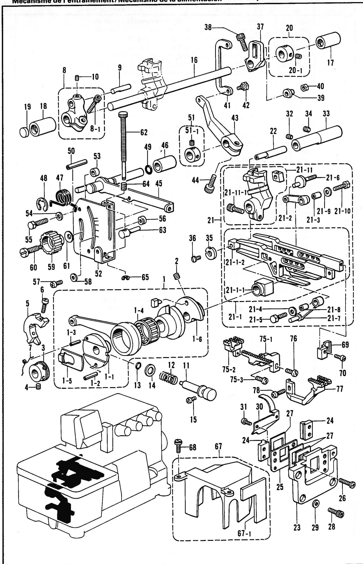
E. 送り関係/Feed mechanism/Transportvorrichtung/
