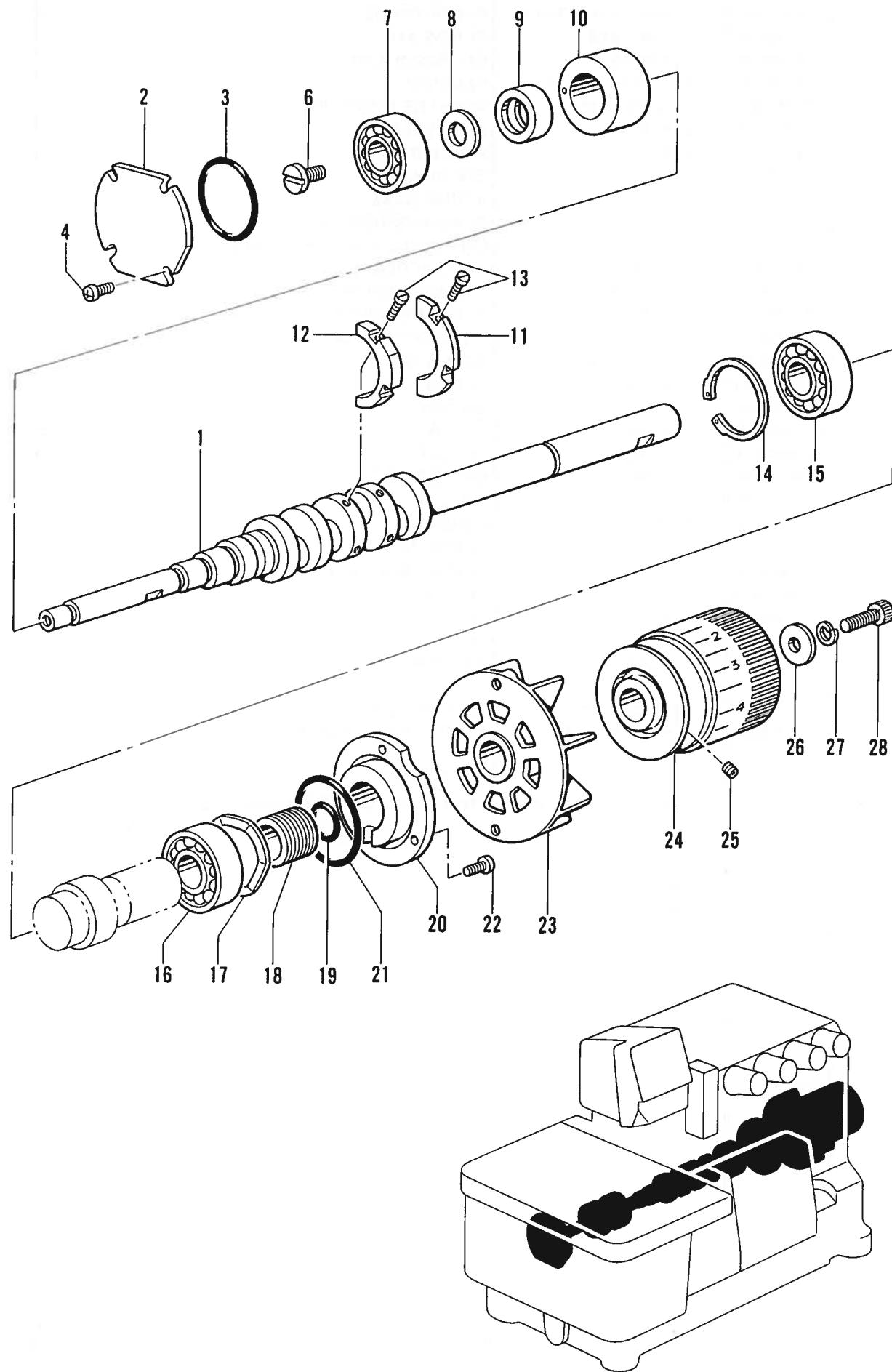
B. 駆動軸関係/Crank shaft mechanism/Kurbelwelle/
