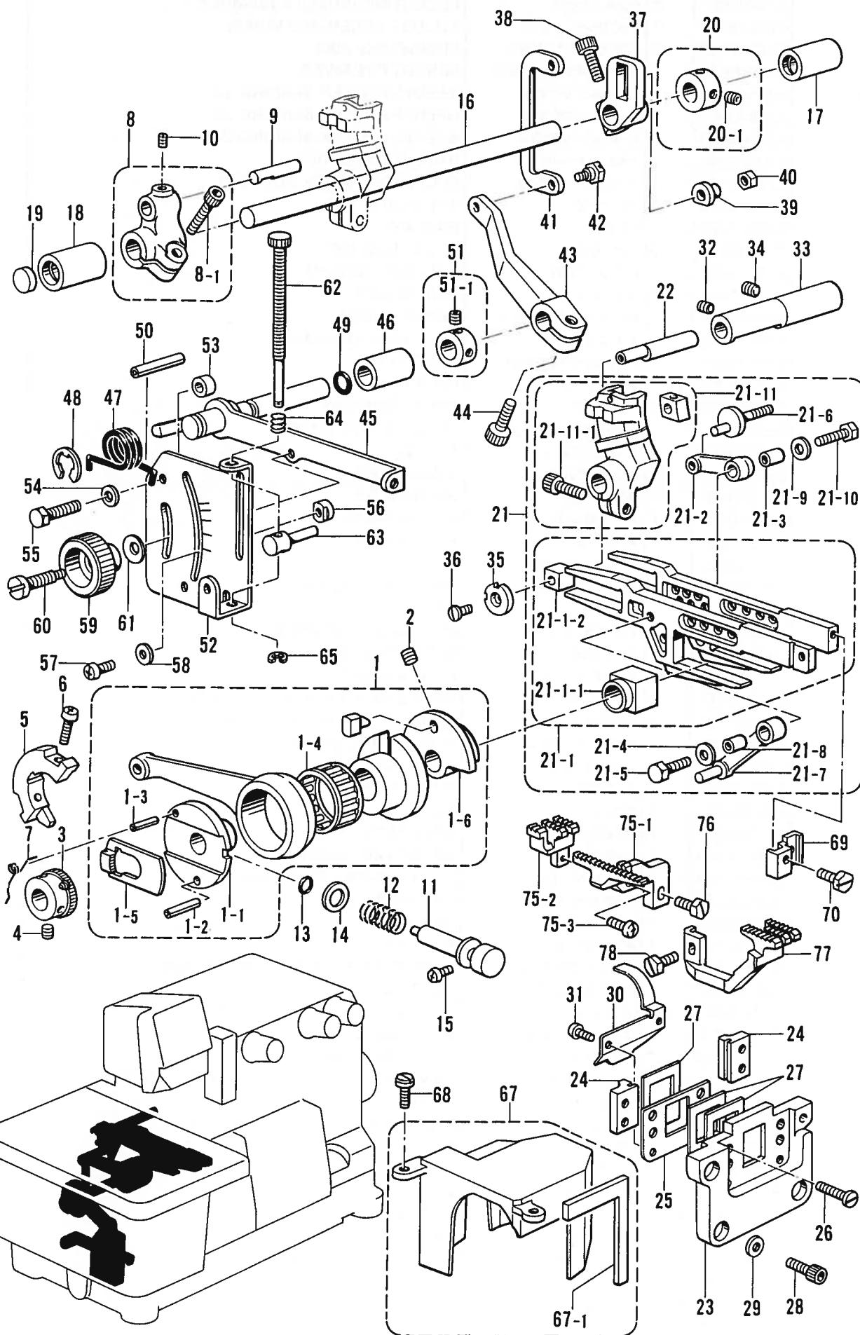
E. 送り関係/Feed mechanism/Transportvorrichtung/
