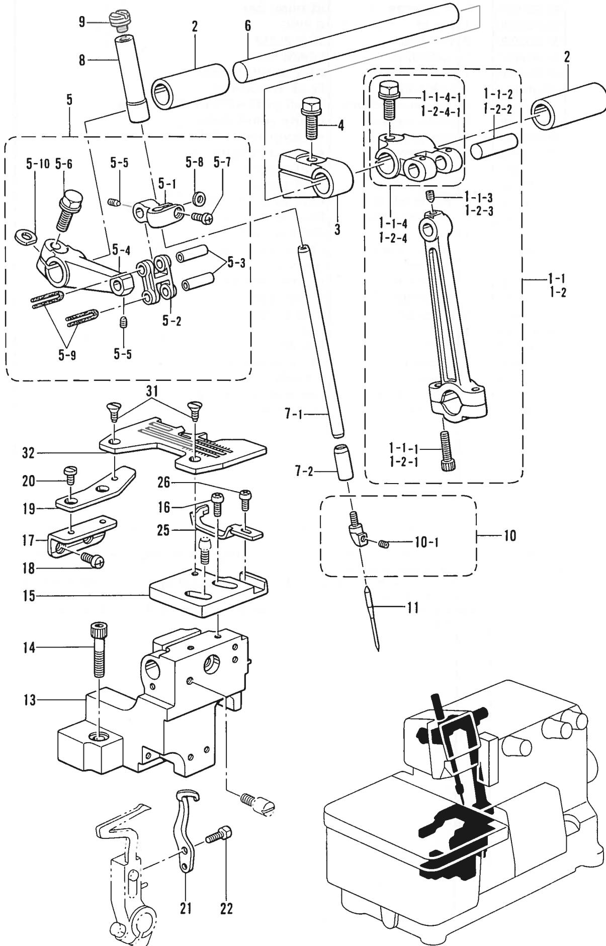
C. 針棒関係 /Needle bar mechanism/Nadelstangenvorrichtung/
