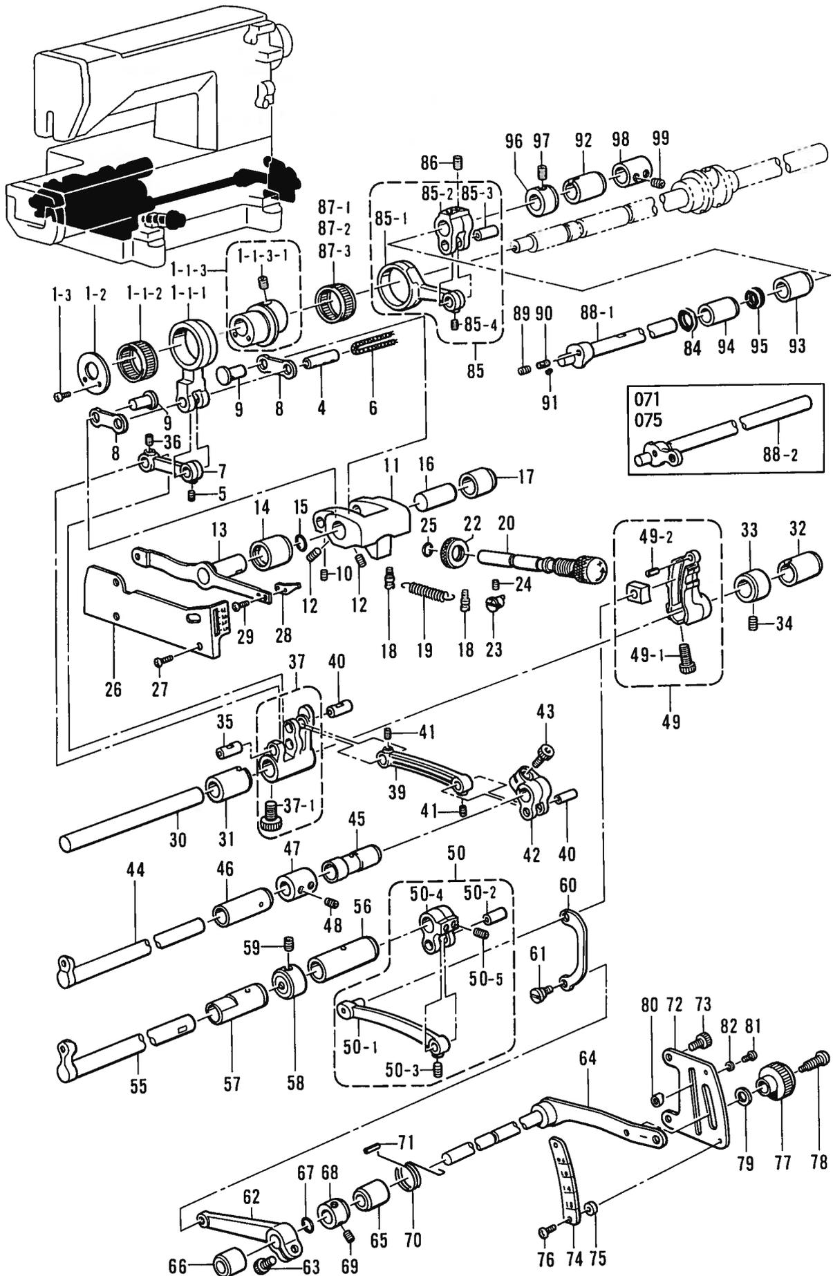
E1. 送り関係 / Feed mechanism/Transportvorrichtung/
