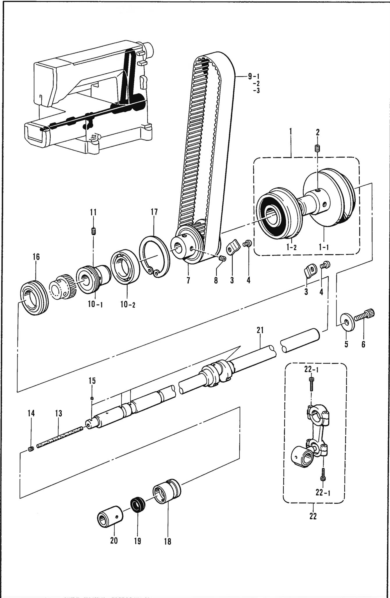
F. 下軸関係/Lower shaft mechanism/Untere Welle/
