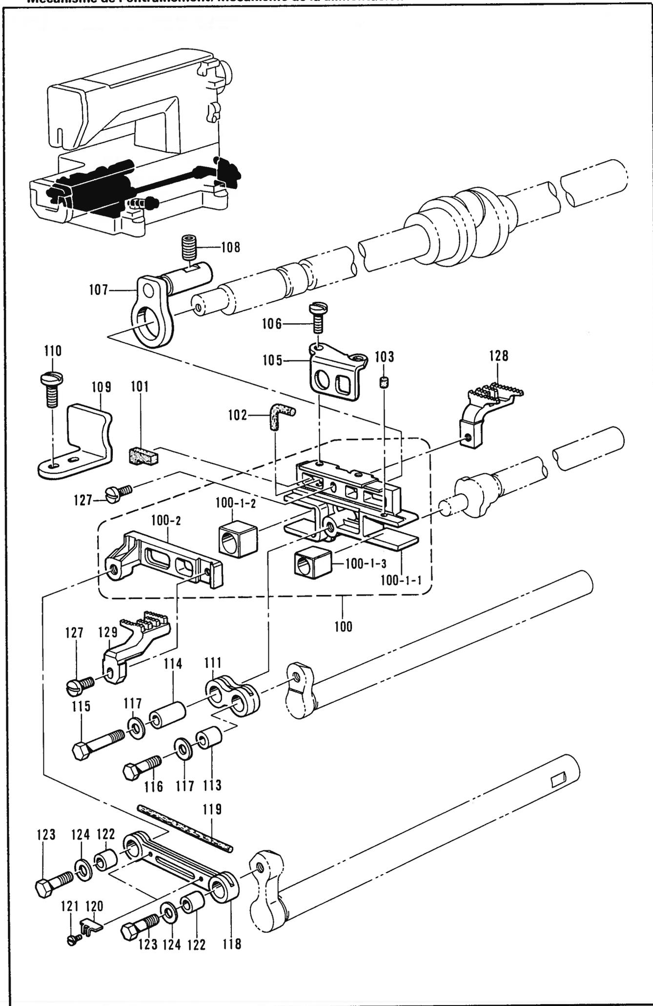
E2. 送り関係/Feed mechanism/Transportvorrichtung/
