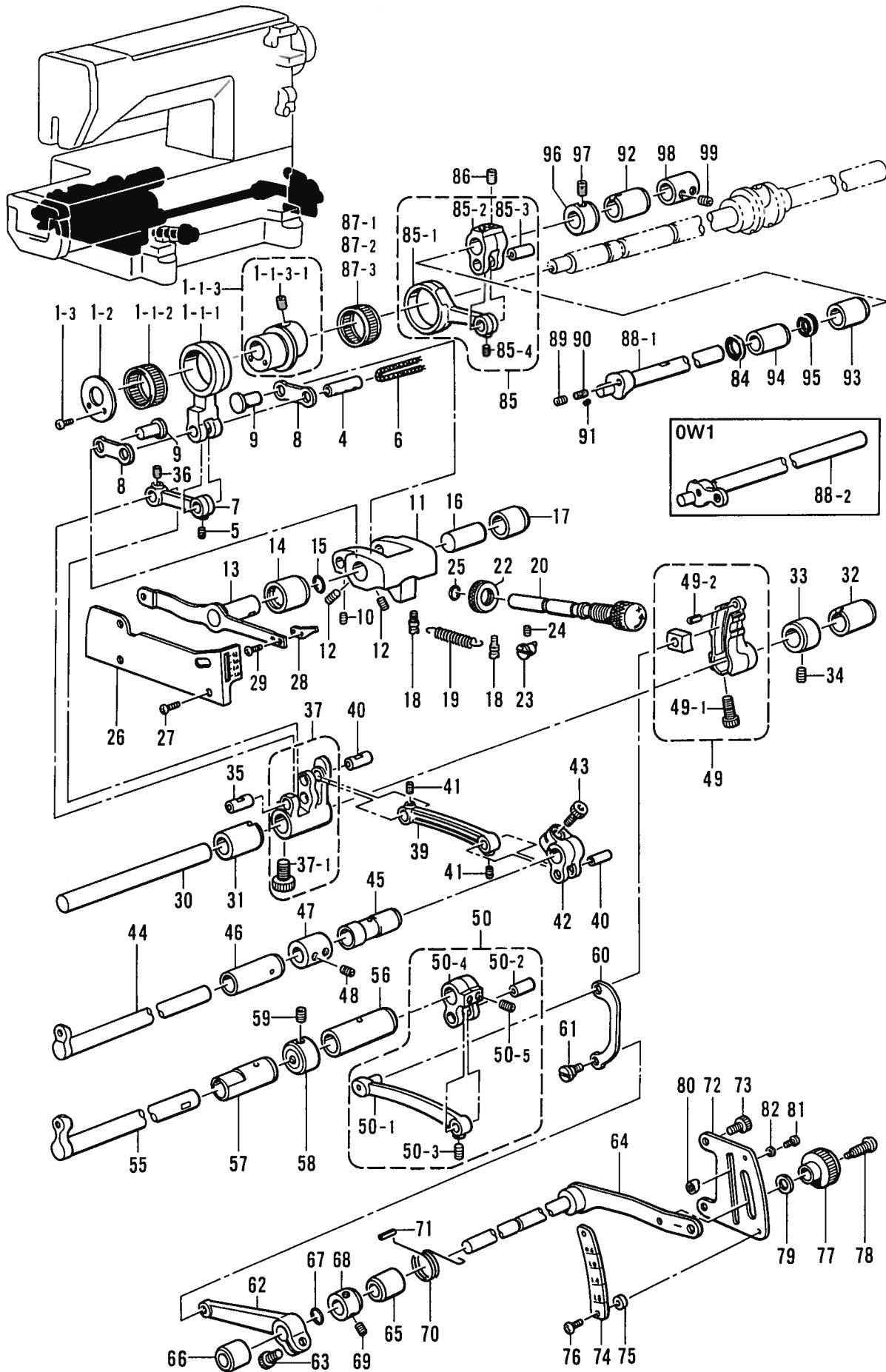
E1. 送り関係/Feed mechanism/Transportvorrichtung/
