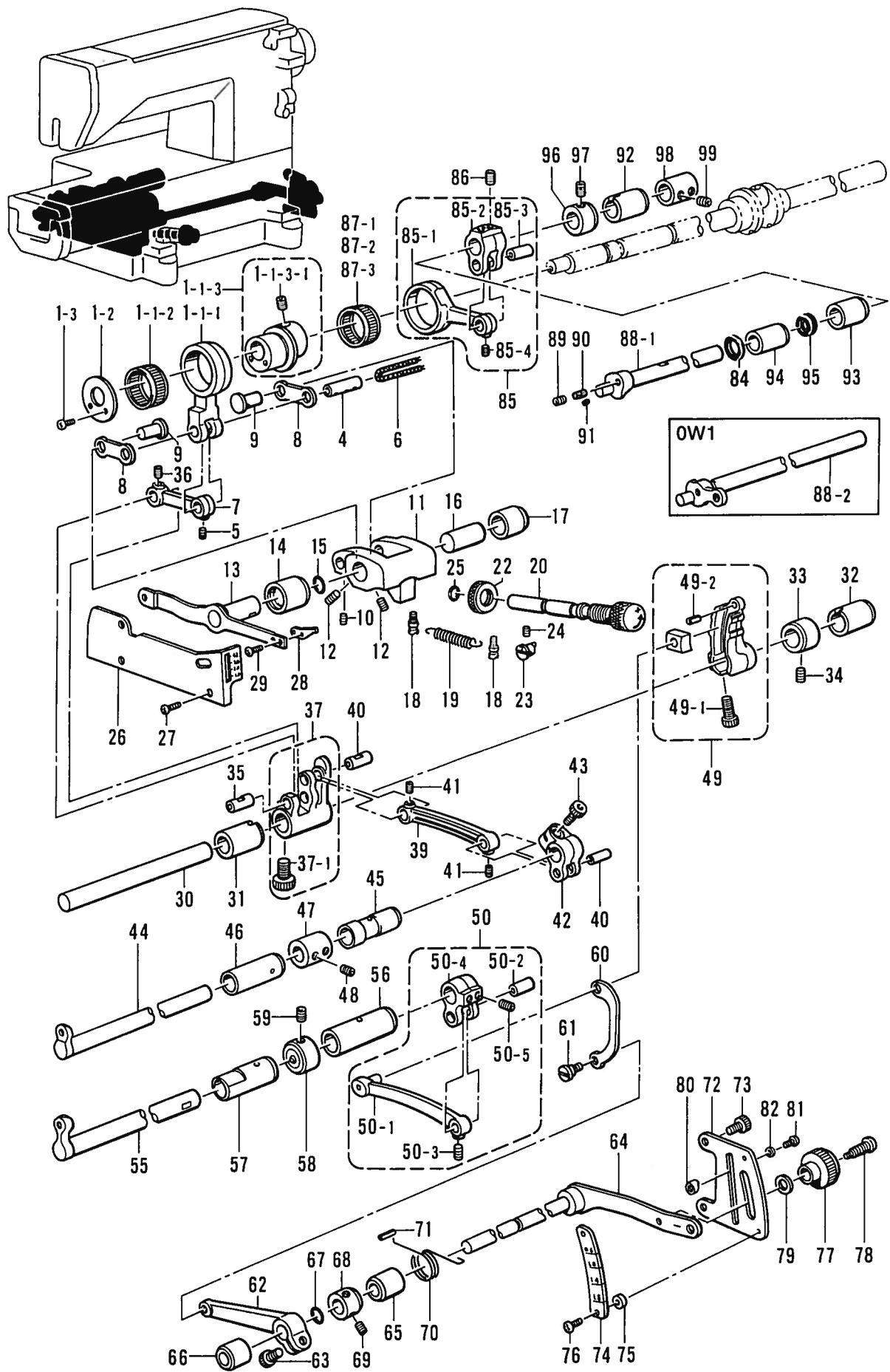
E1. 送リ関係/Feed mechanism/Transportvorrichtung/
