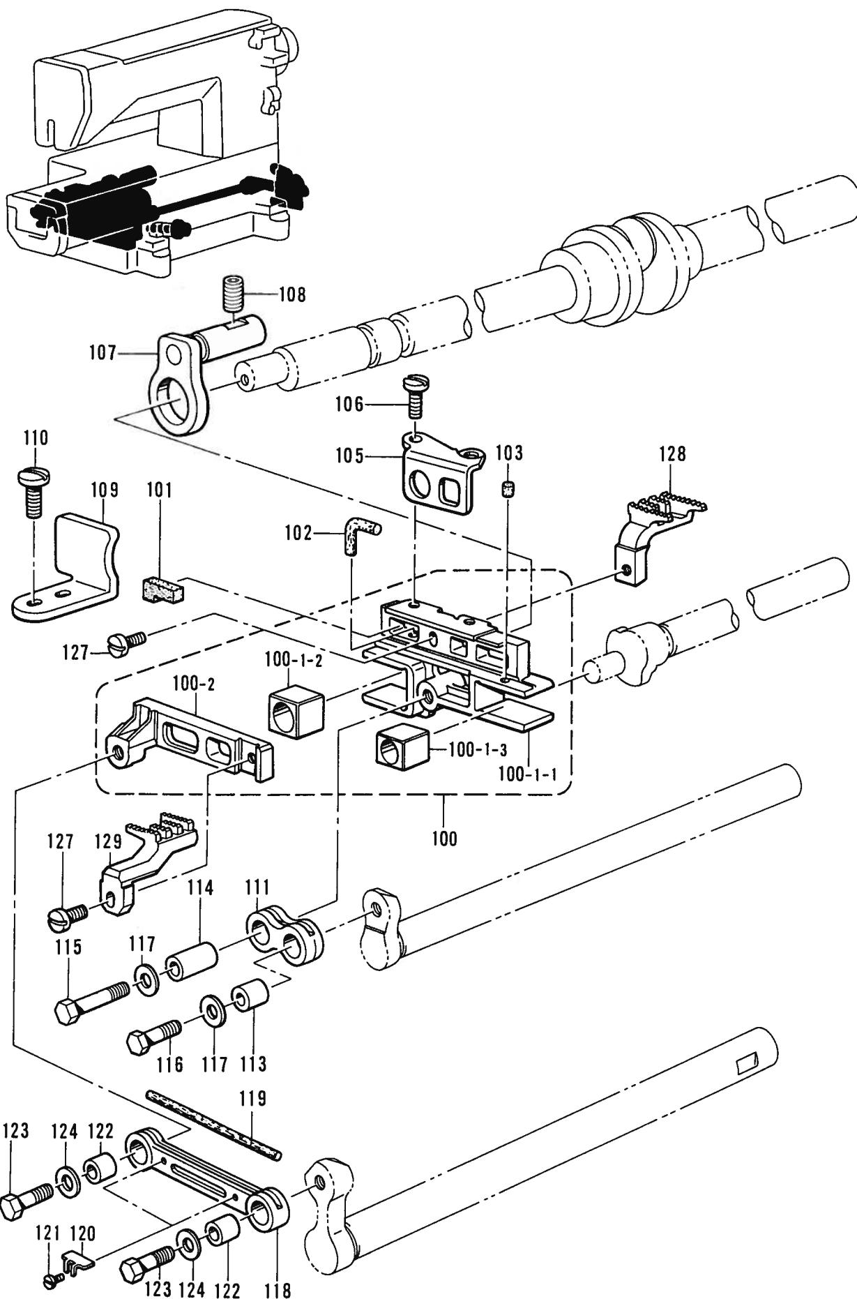
E2. 送り関係/Feed mechanism/Transportvorrichtung/
