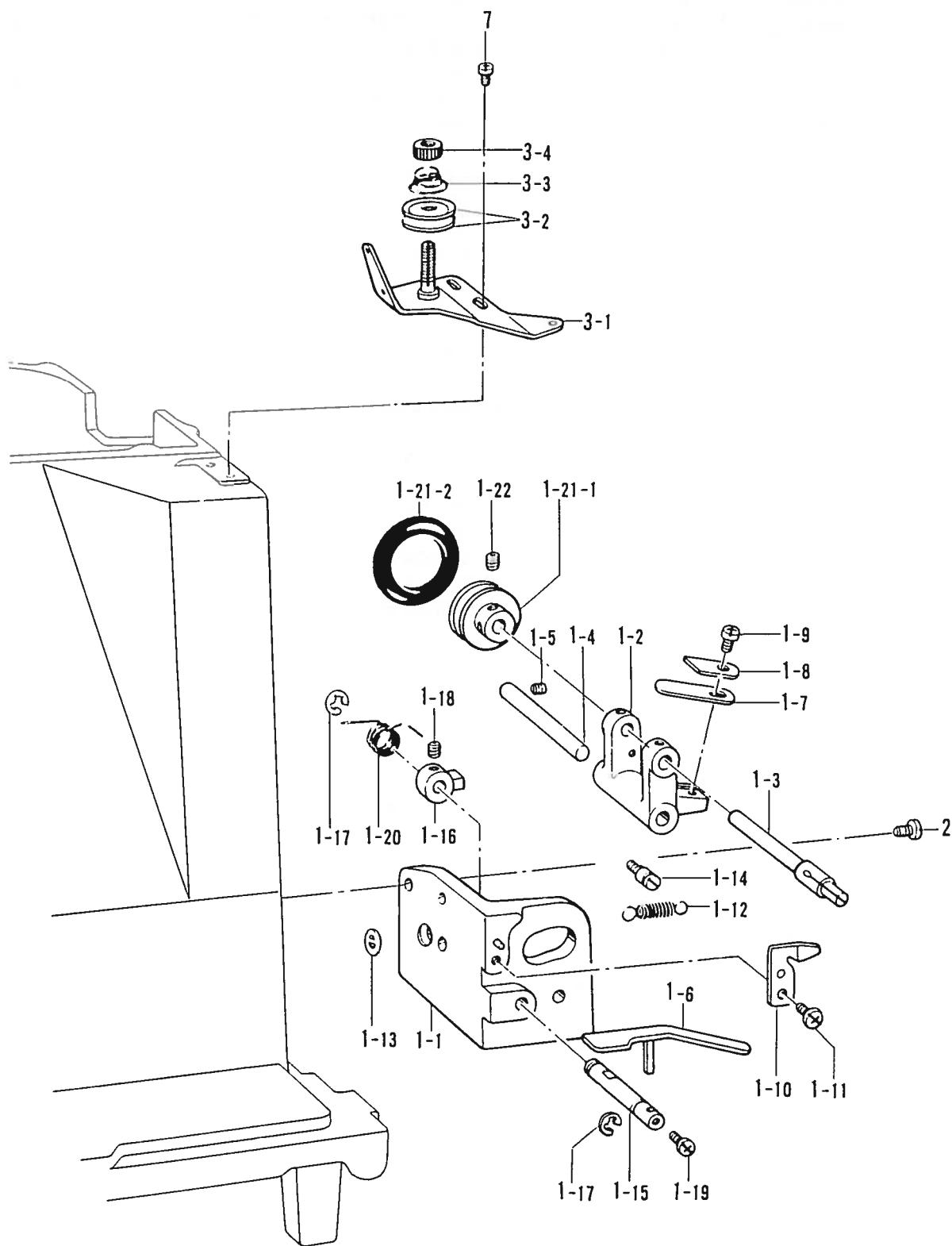
L. 糸巻キ関係/Bobbin winder mechanism/Spuler/
