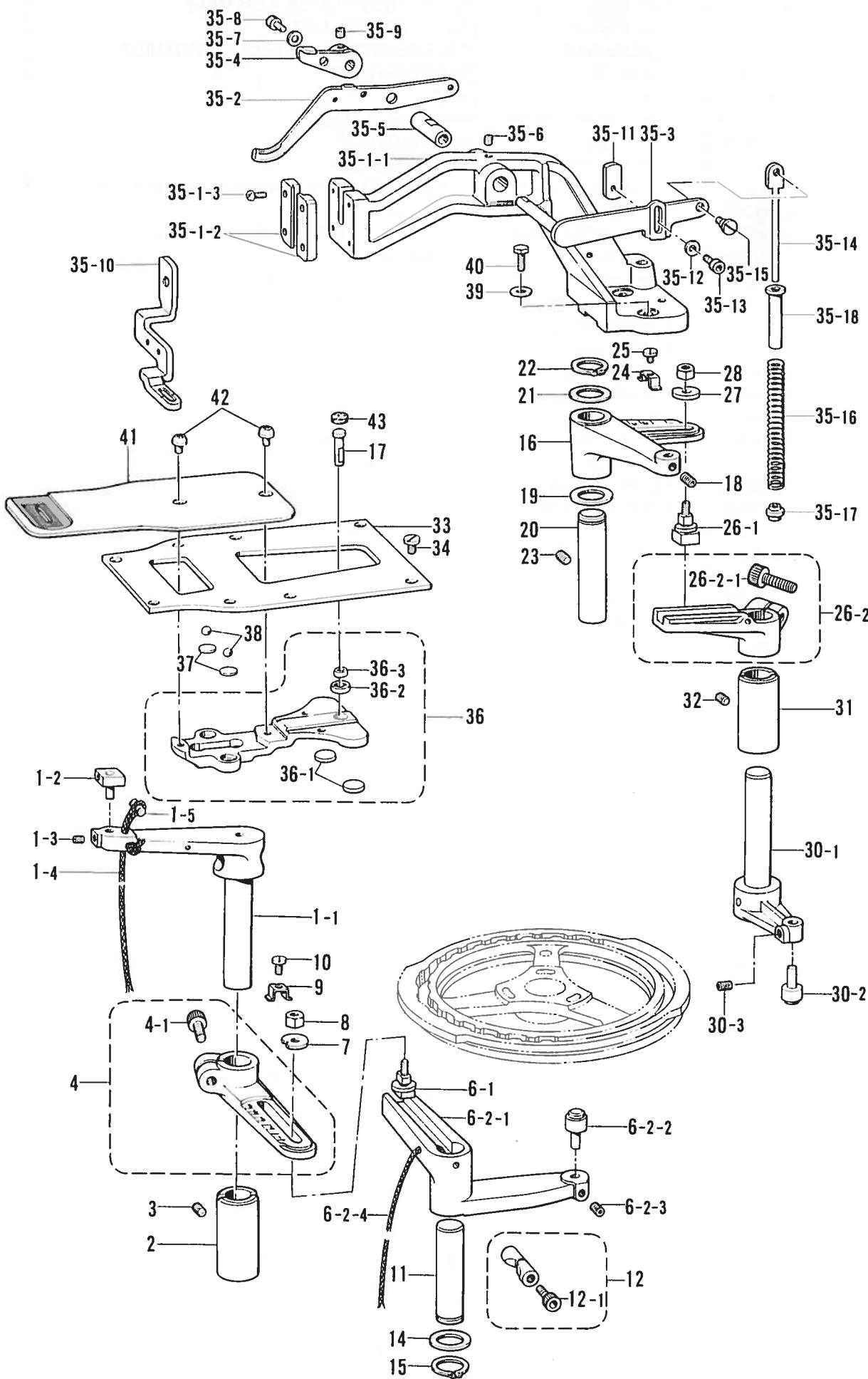
D. 送り関係/Feed mechanism/Transportvorrichtung/
