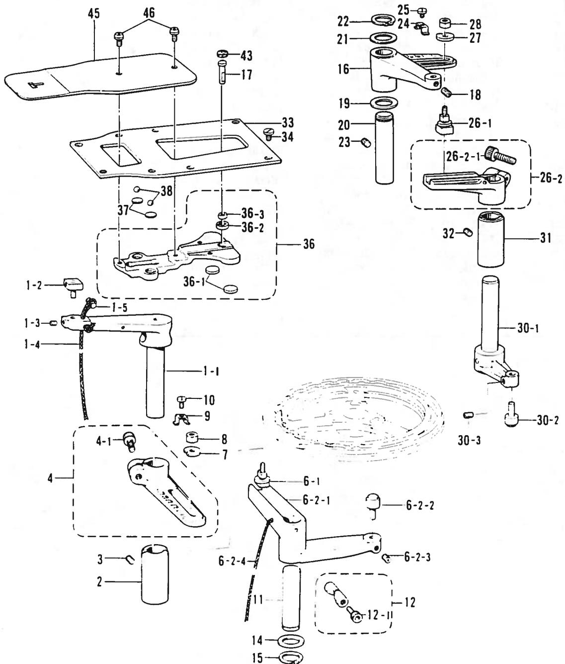
E1. 送り関係 /Feed mechanism/Transportvorrichtung/
