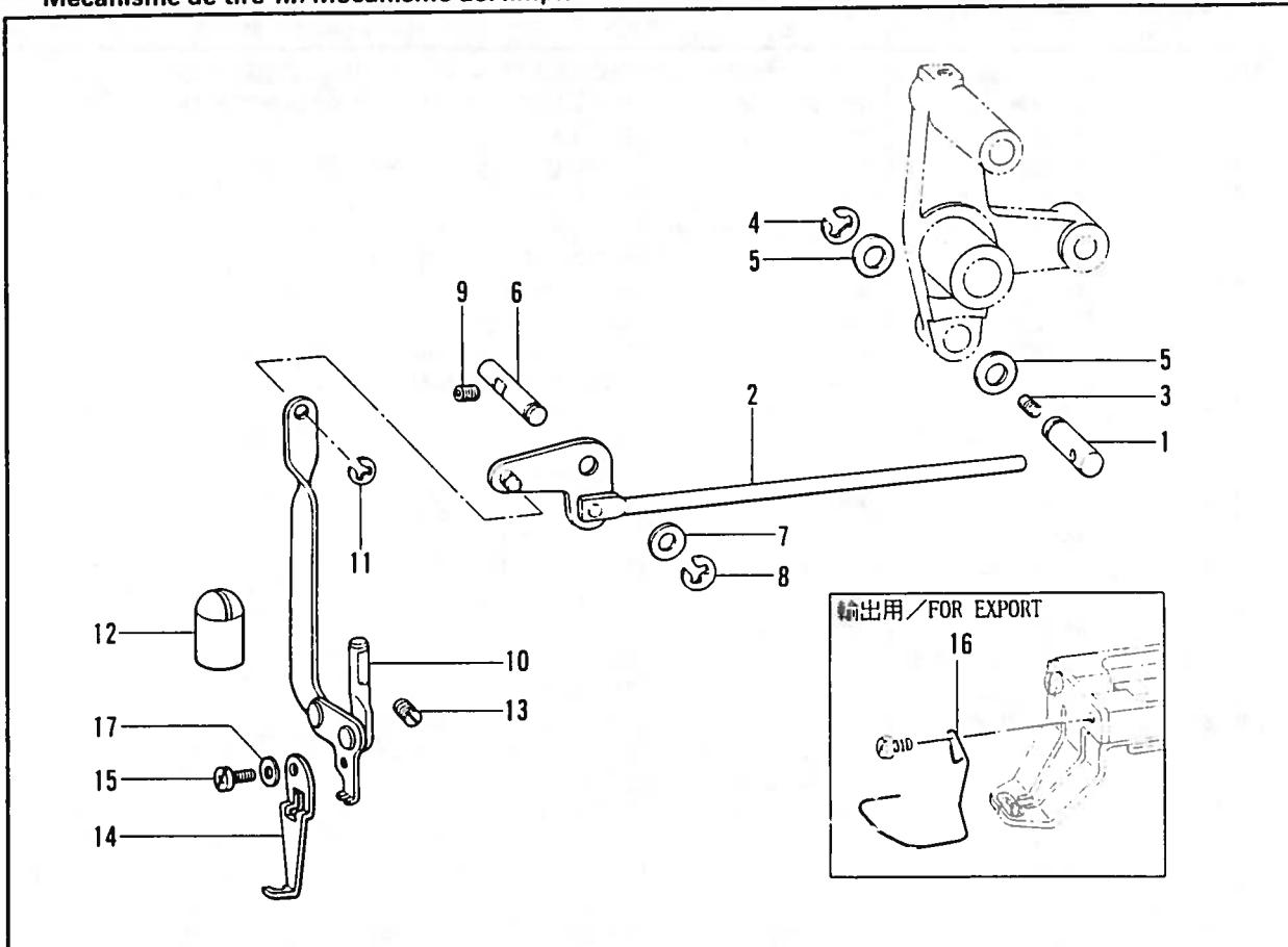
Q. 糸締め関係 / Thread nipper mechanism / Fadenspannvorrichtung /
