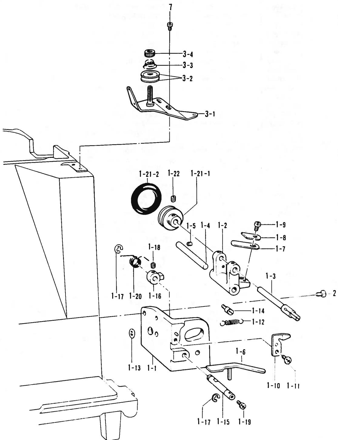
M. 糸巻キ関係 / Bobbin winder mechanism / Spuler /
