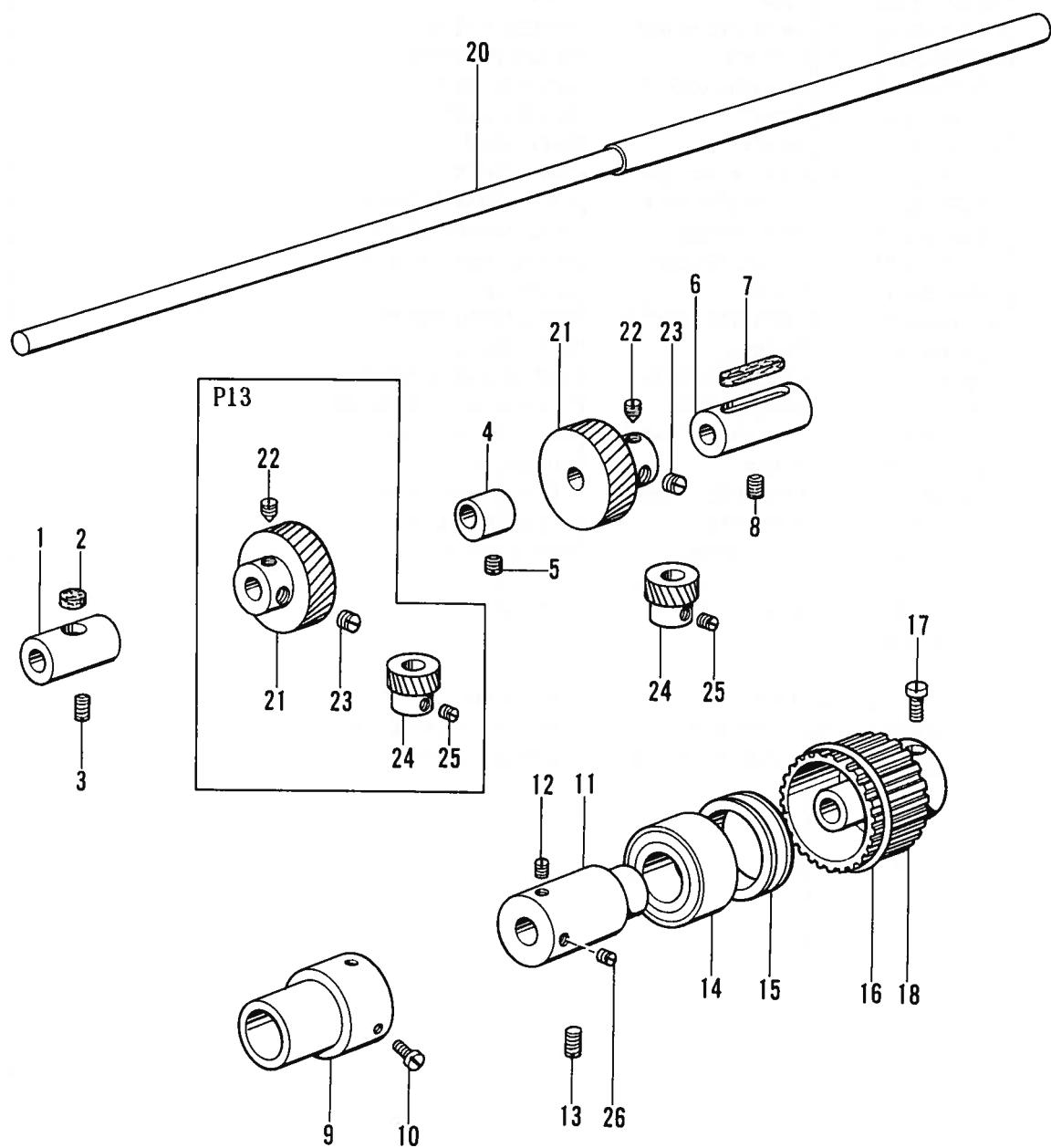
G. 下軸関係 /Lower shaft mechanism/Untere Welle/
