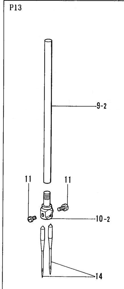
C. 針棒関係/Needle bar mechanism/Nadelstangenvorrichtung/
