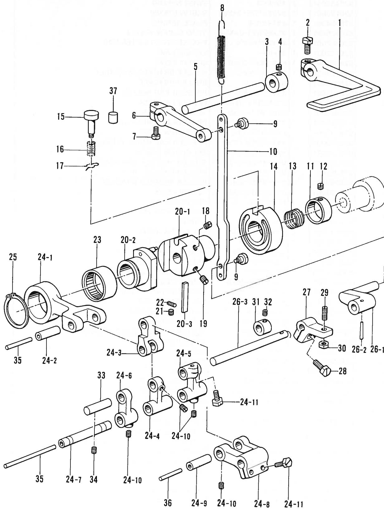
E. 送り関係 / Feed mechanism/Transportvorrichtung/
