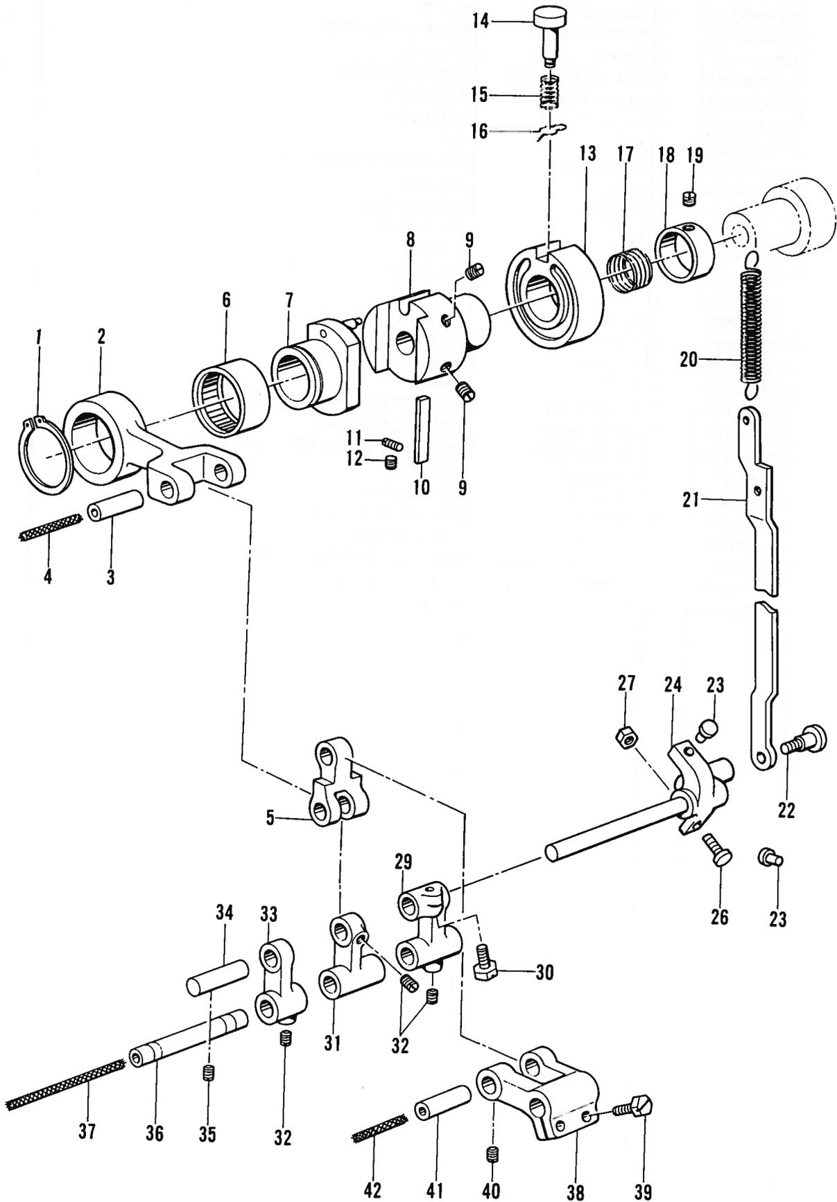
F. 送り関係/Feed mechanism/Transportvorrichtung/
