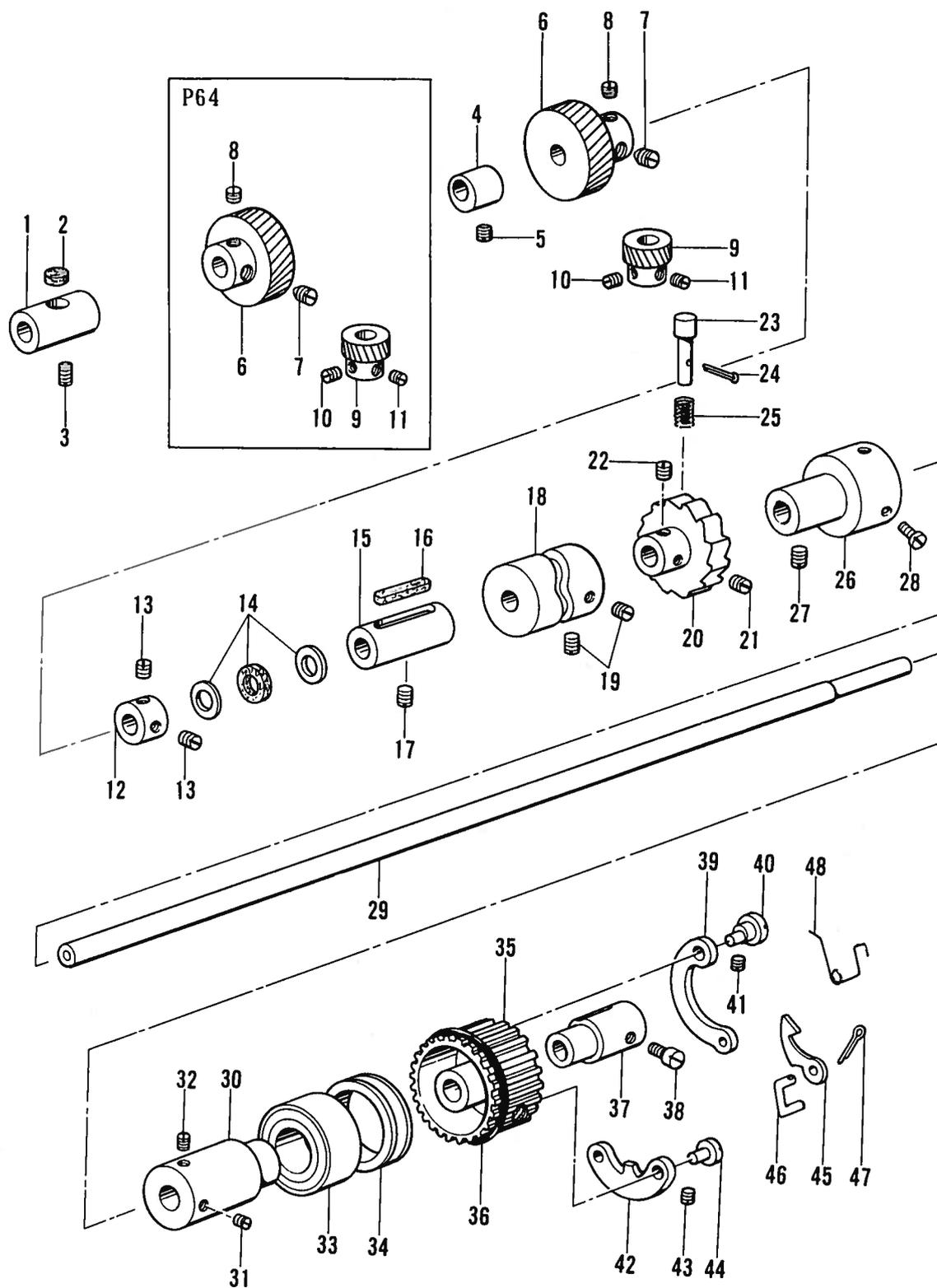
H. 下軸関係/Lower shaft mechanism/Untere Welle/
