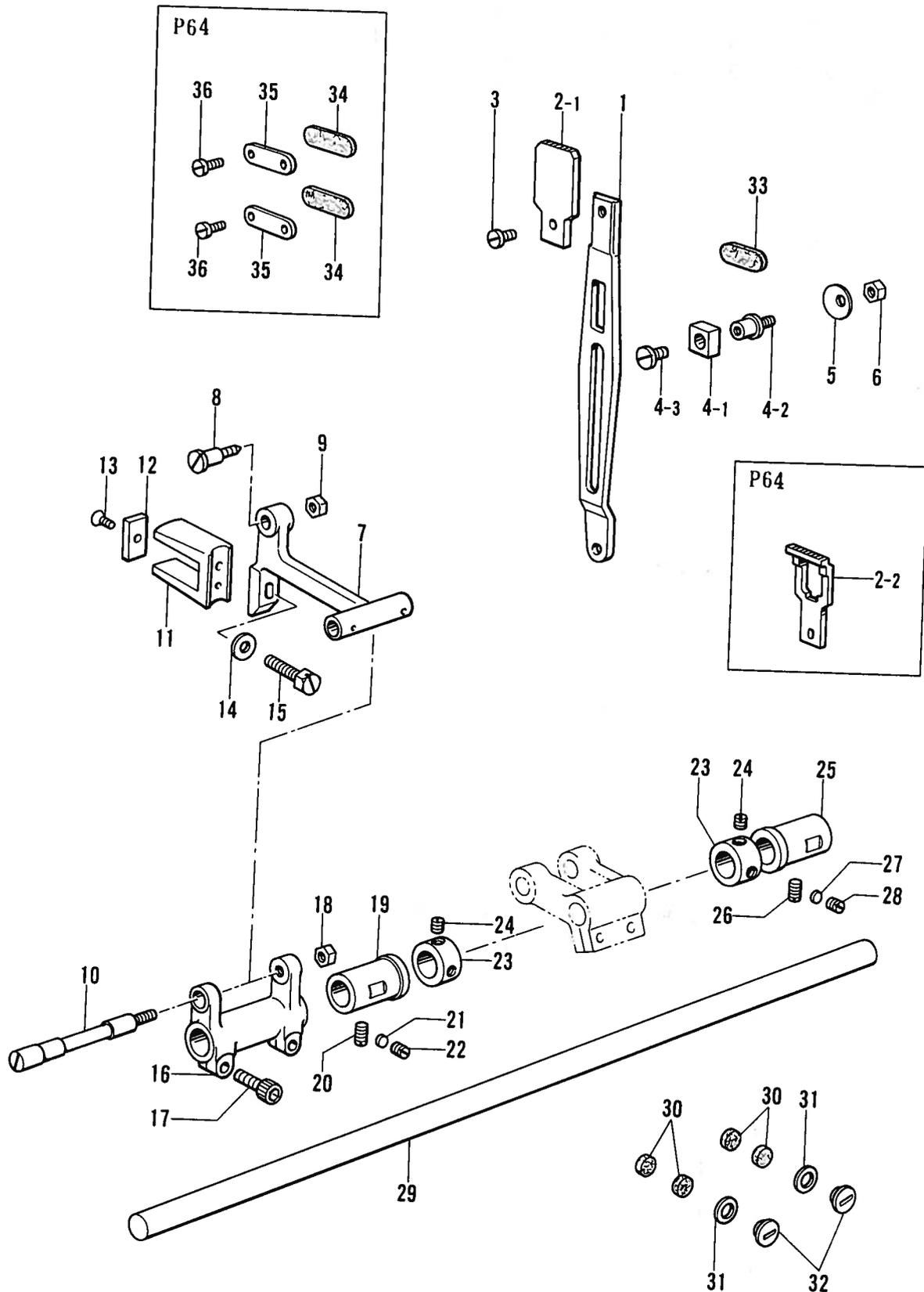
G. 送り軸関係/Feed shaft mechanism/Transport welle/
