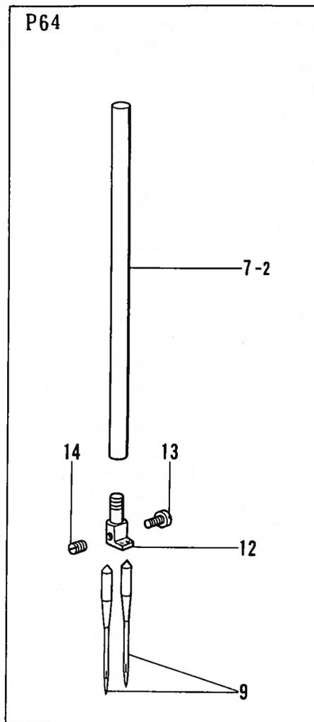
C. 針棒関係/Needle bar mechanism/Nadelstangenvorrichtung/
