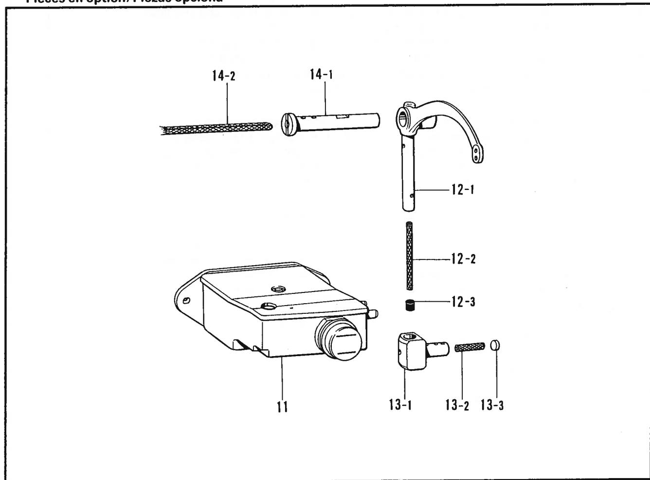
J. 下軸関係/Lower shaft mechanism/Untere welle/
