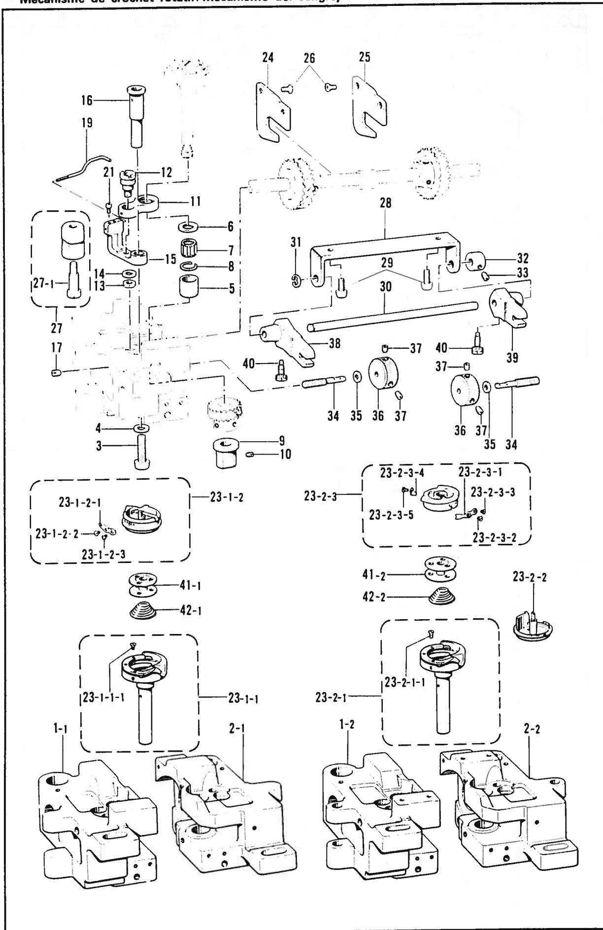
K. カマ関係/Rotary hook mechanism/Greifervorrichtung/
