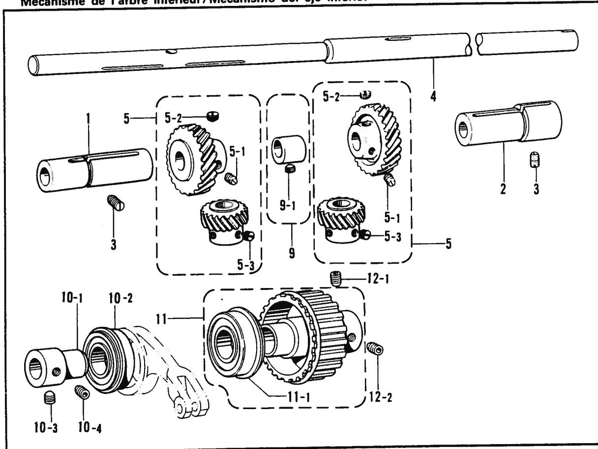
H. 逆転関係 (糸切り) / Quick reverse mechanism (Thread Trimmer) / Umkehr (Fadenabschneider) /
