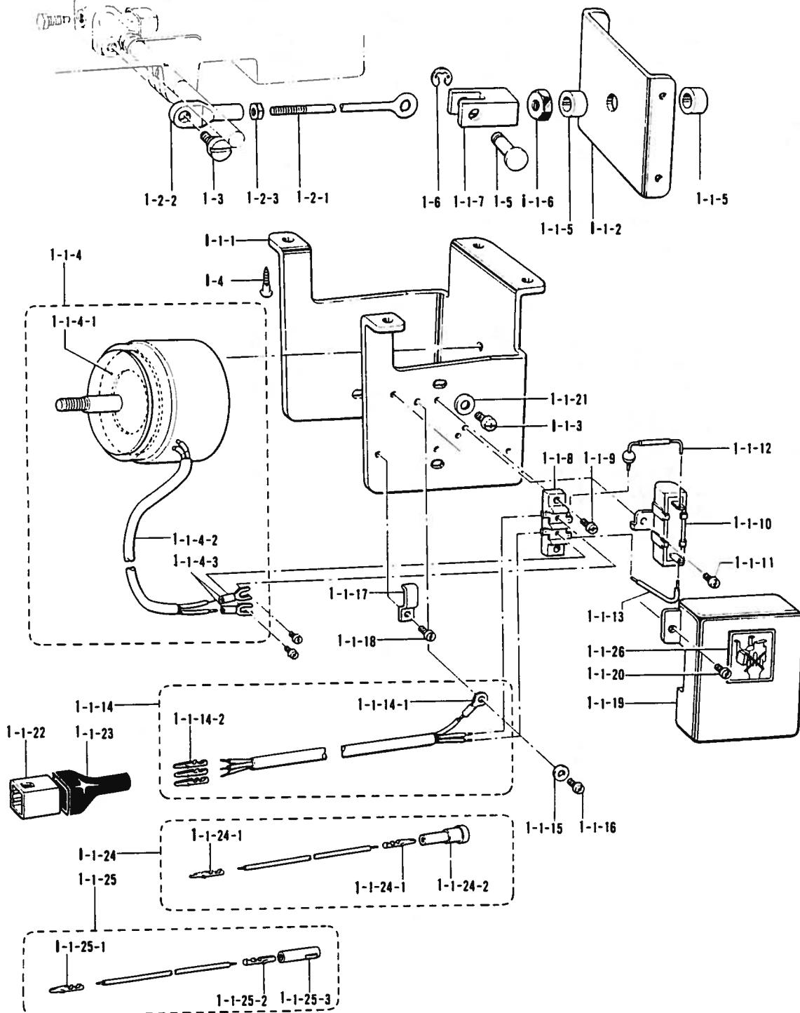
V1. 電磁押工上ヶ関係 / Presser foot lifting solenoid set /
