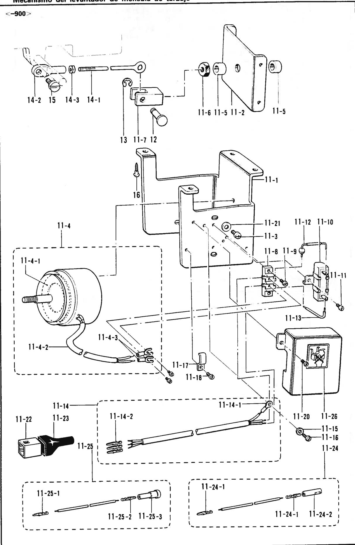
G2. 押工上部関係/Work clamp lifter mechanism/
