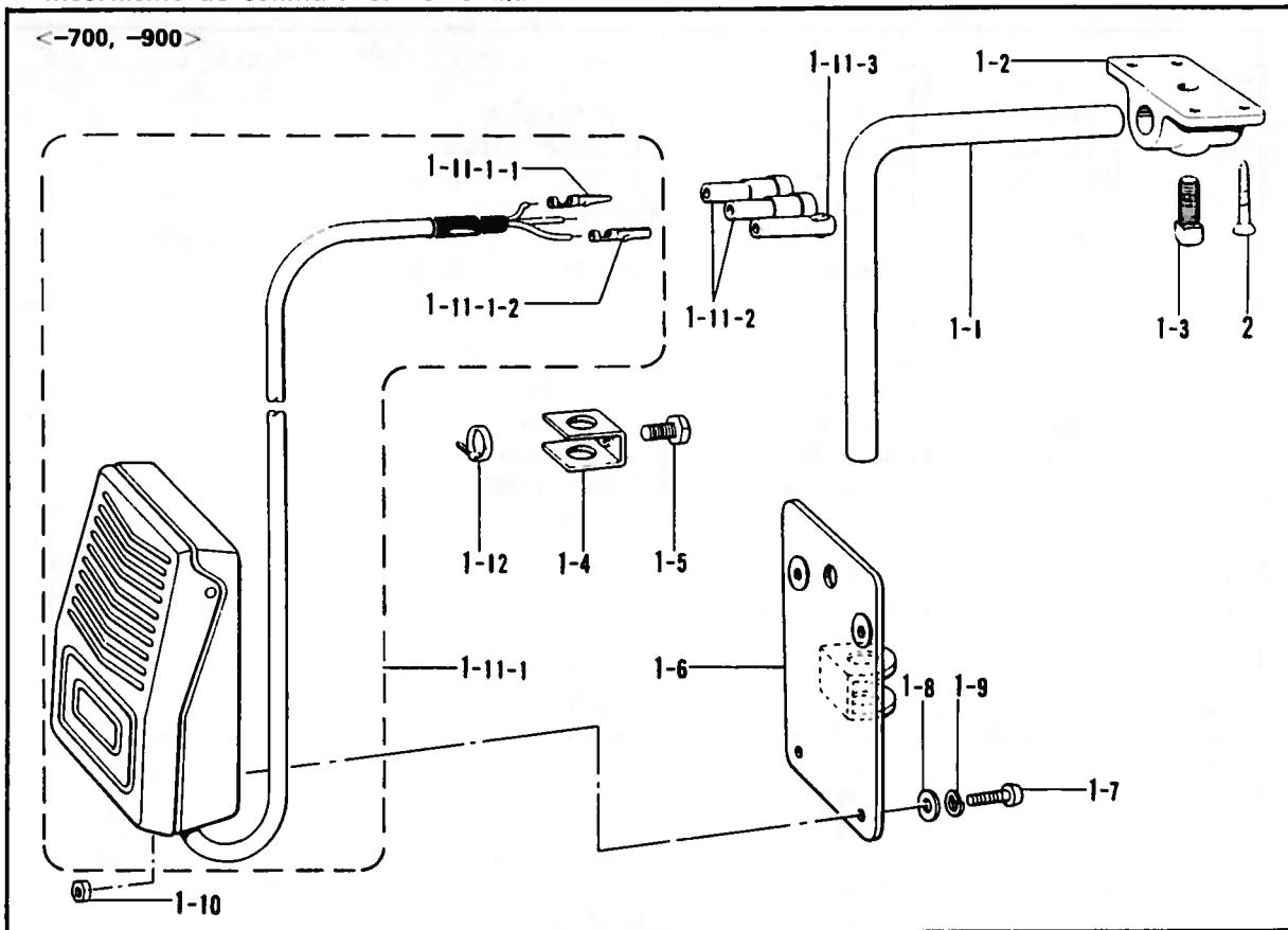
T. 逆転スイッチ関係 (糸切り) / Quick reverse switch mechanism (Thread Trimmer) /
