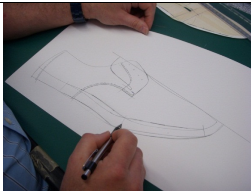
A lining standard with the adding allowances
