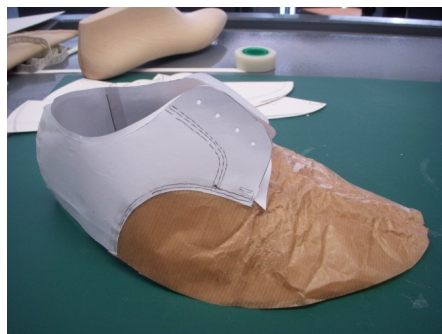
Complete paper simulation before board pattern making
